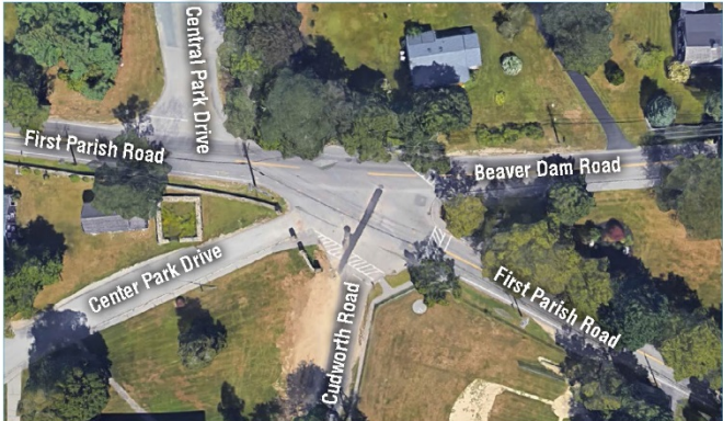
Cudworth Road’s intersection with First Parish Road is not only a 6 way intersection, the visibility is poor and the right of way is not clear. This is a major intersection for cars exiting the Senior Center in Option A. A cost has been included to restructure the intersection marginally.
