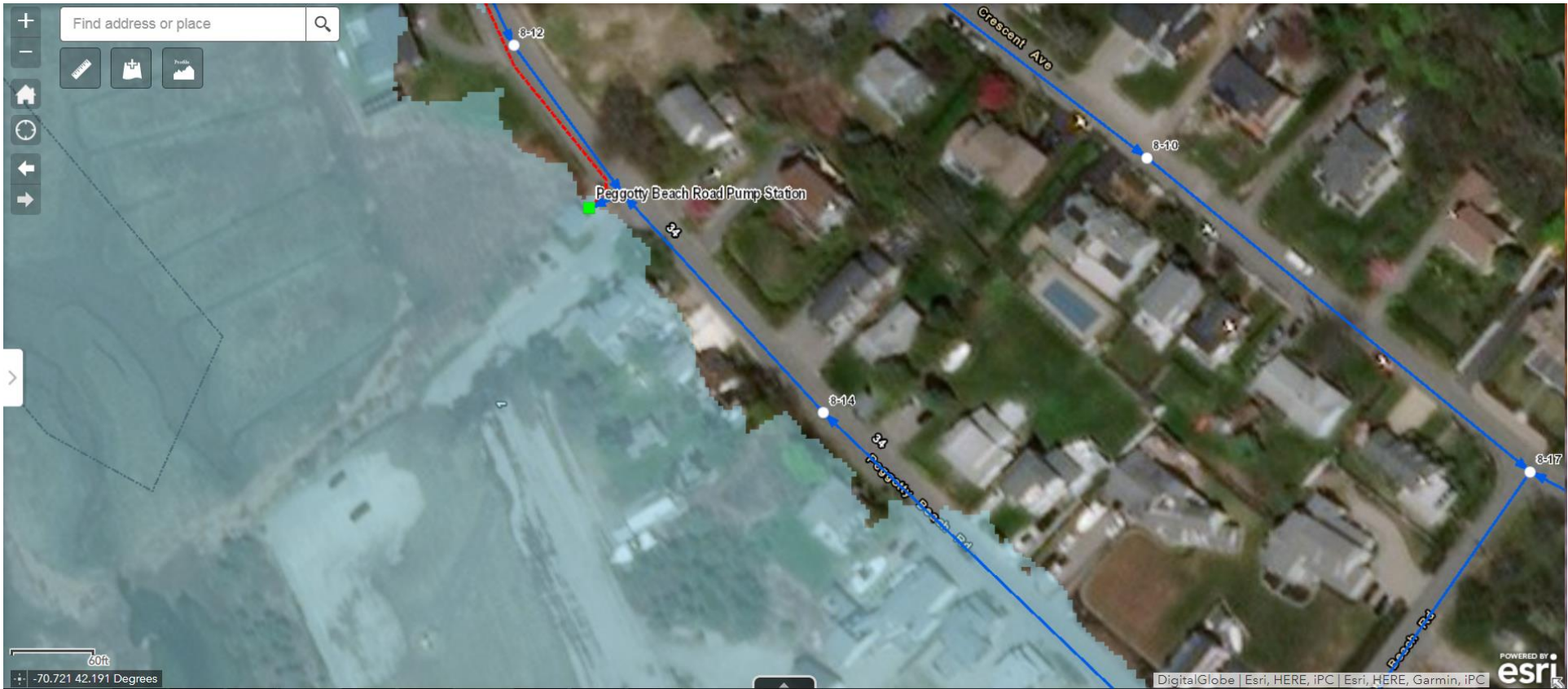
Figure 4-40: Flood Inundation at Peggotty Beach Pump Station (Floodwater = 11 feet NAVD88)
