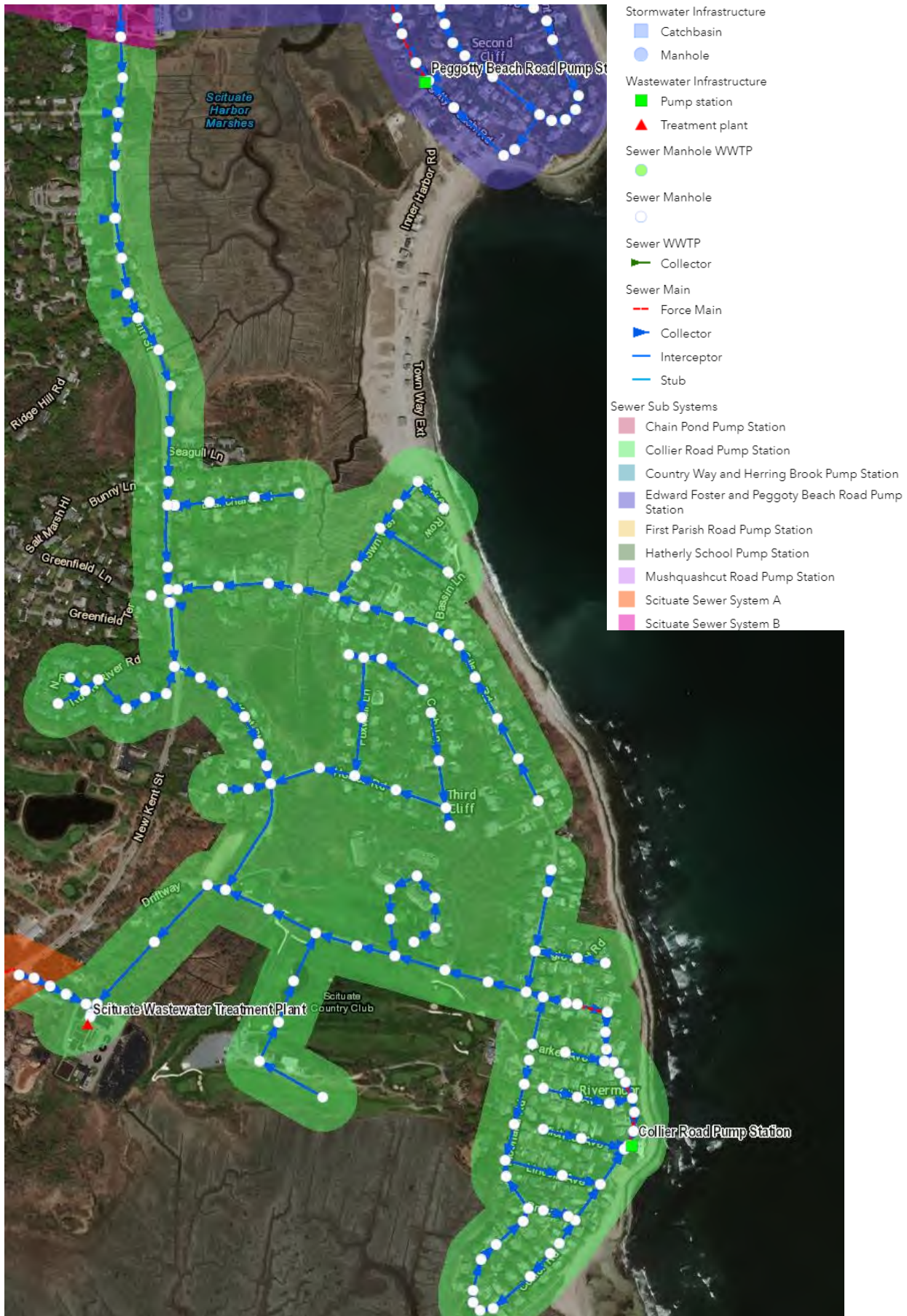
Figure 2-5: Collier Road Pup Station Sewer System
