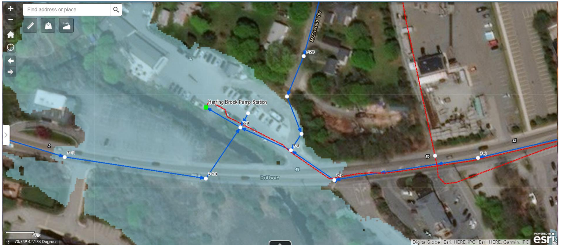
Figure 4-35: Flood Stillwater Inundation (Stillwater = 15 feet NAVD88)
