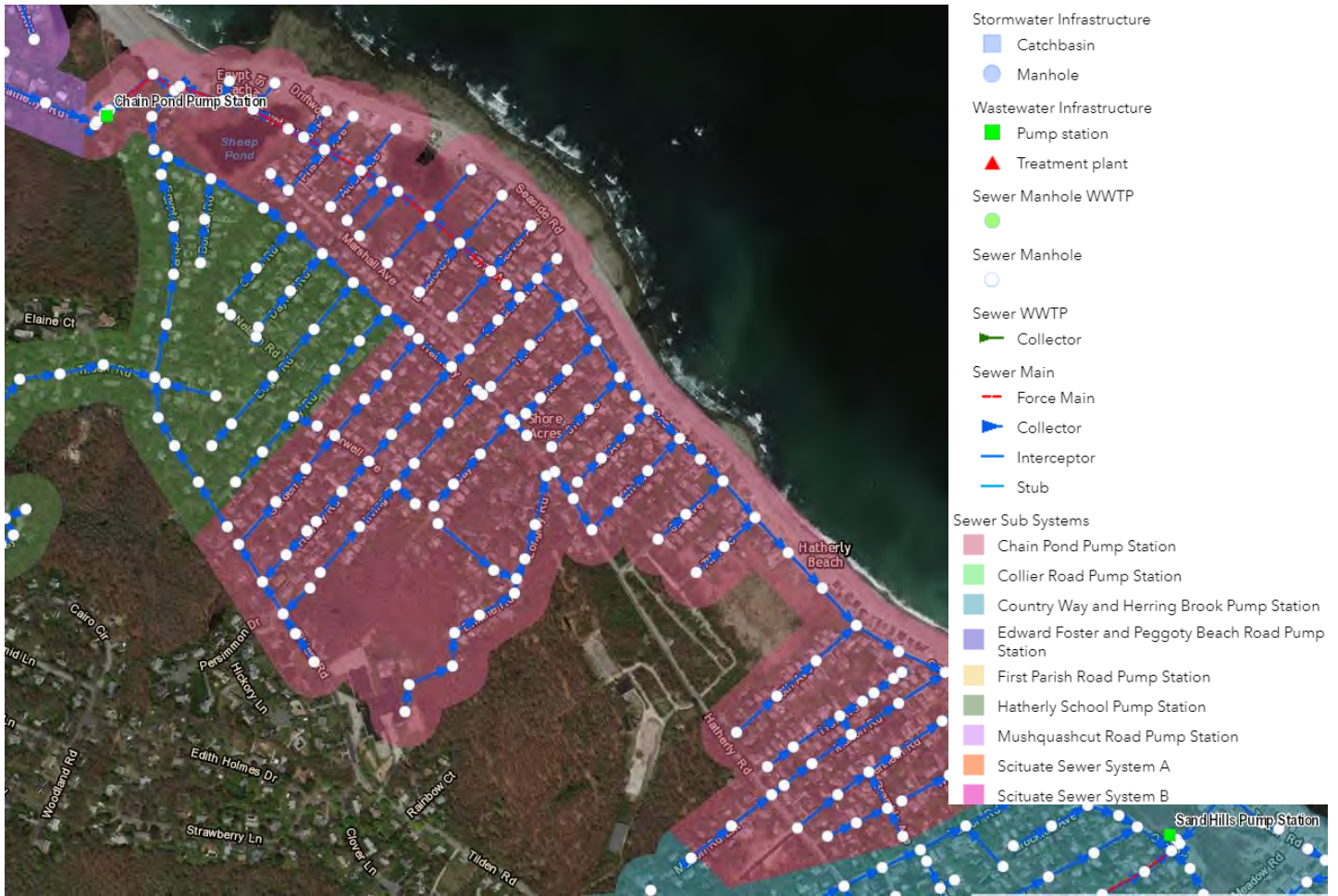
Figure 2-3: Chain Pond Pump Station Sewer System
