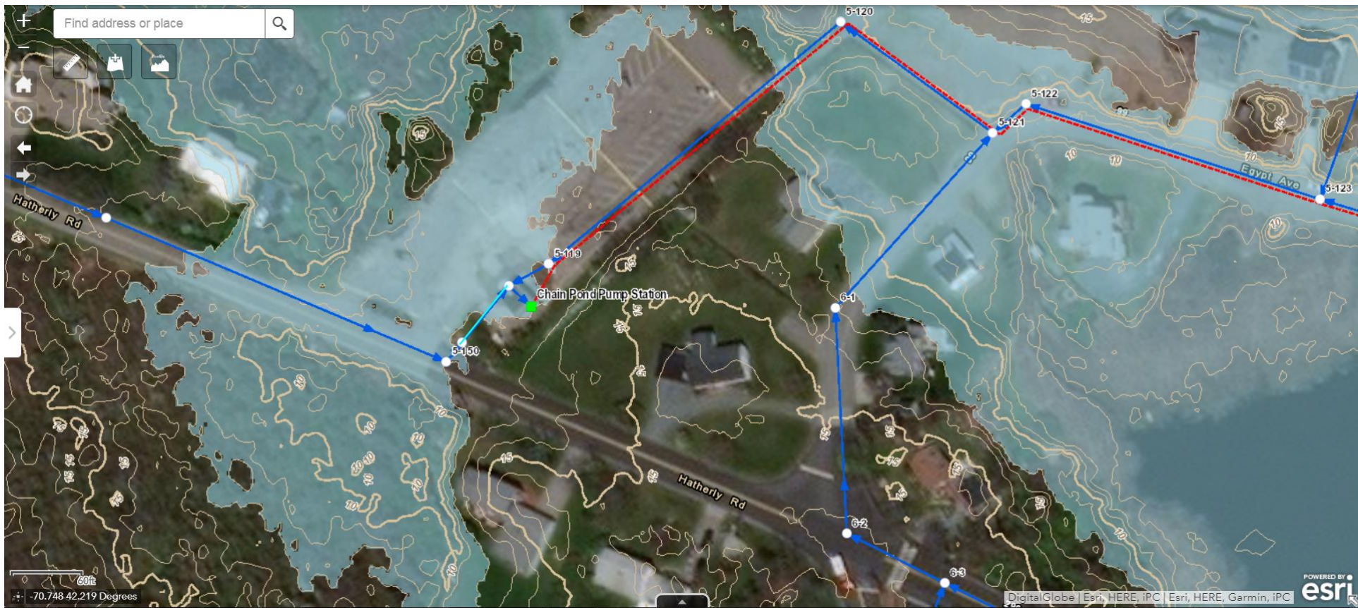
Figure 4-51: Flood Inundation at Chain Pond Pump Station (Floodwater = 12 feet NAVD88)
