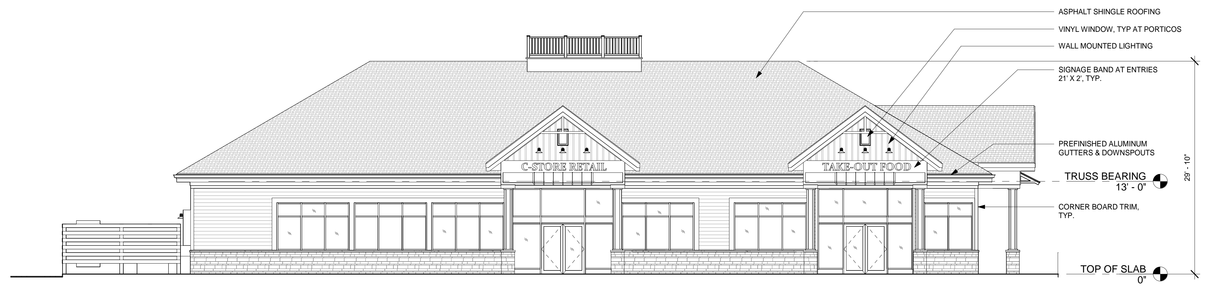
NORTH ELEVATION (NEW DRIFTWAY SIDE) 1/8" = 1'-0" 1
