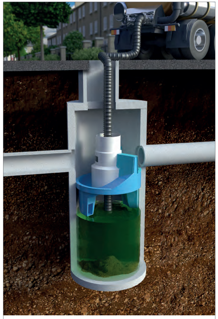
Fig.4 Floatables are removed with a vactor hose
