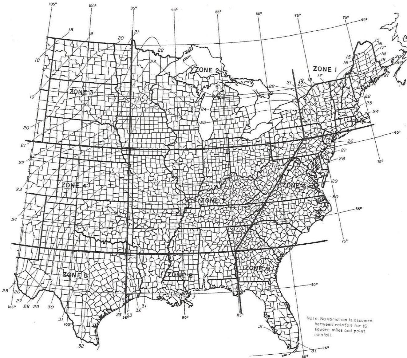
Figure 15. Probable maximum precipitation (inches) east of the 105° meridian for an area of 10 square miles and 6 hours' duration. 288-D-2449A, 288-D-2754, 288-D-2755.
