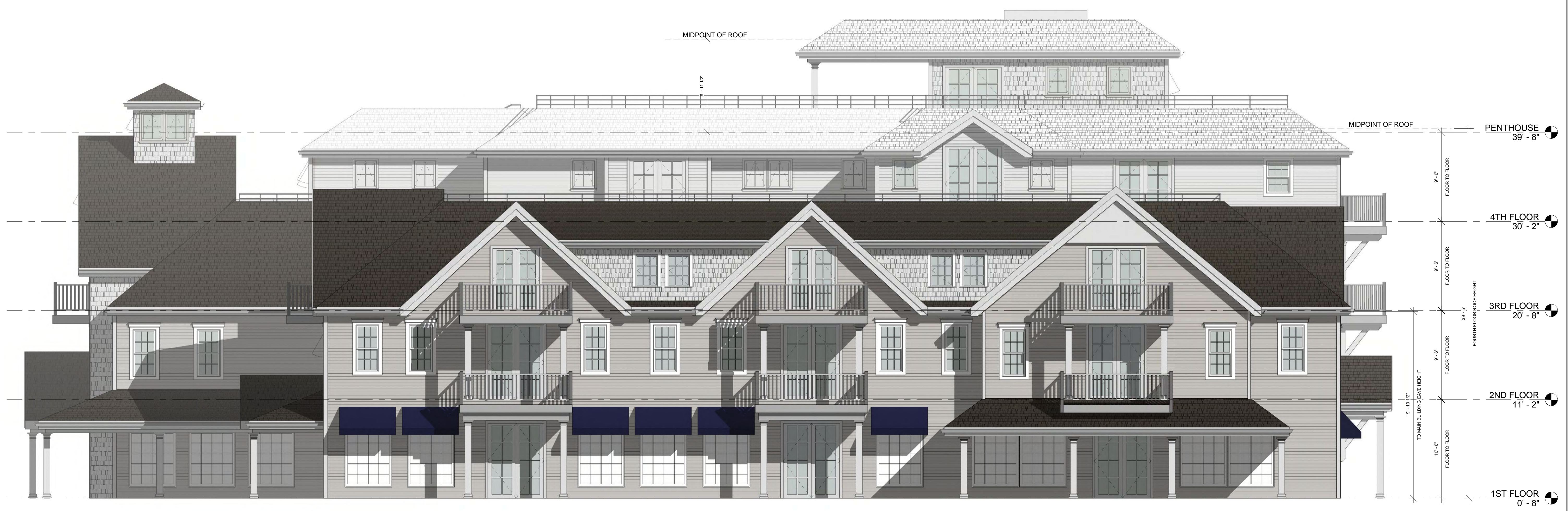
① FRONT ELEVATION (DRIFTWAY) 3/16" = 1'-0"
