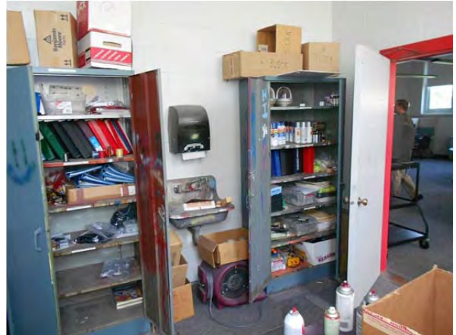
Paint storage should be away from combustibles and stored in approved cabinets.
