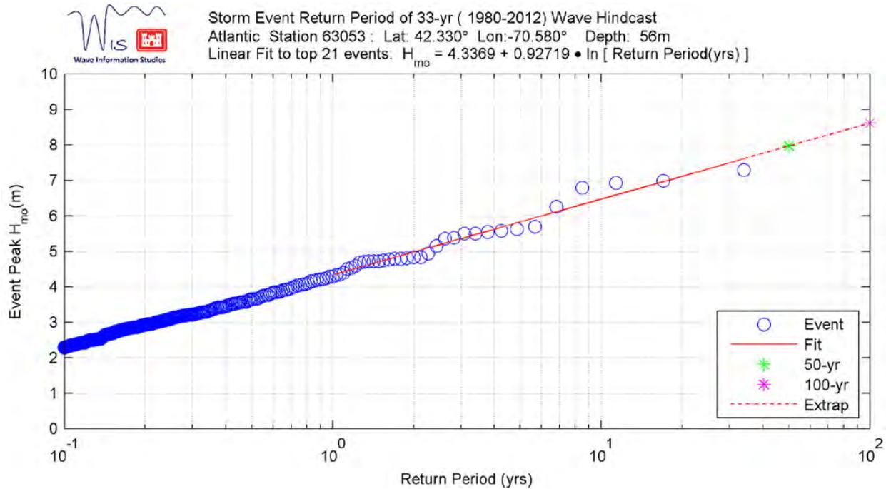
Figure 3.8 WIS hindcast station 63053 extreme analysis plot for significant wave height.
