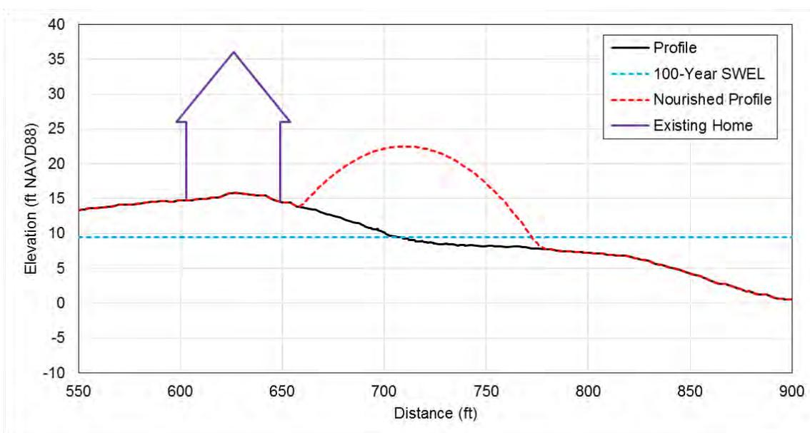
Figure 7.56 Schematic of the proposed dune profile required to satisfy the “540 rule” along Humarock South.
