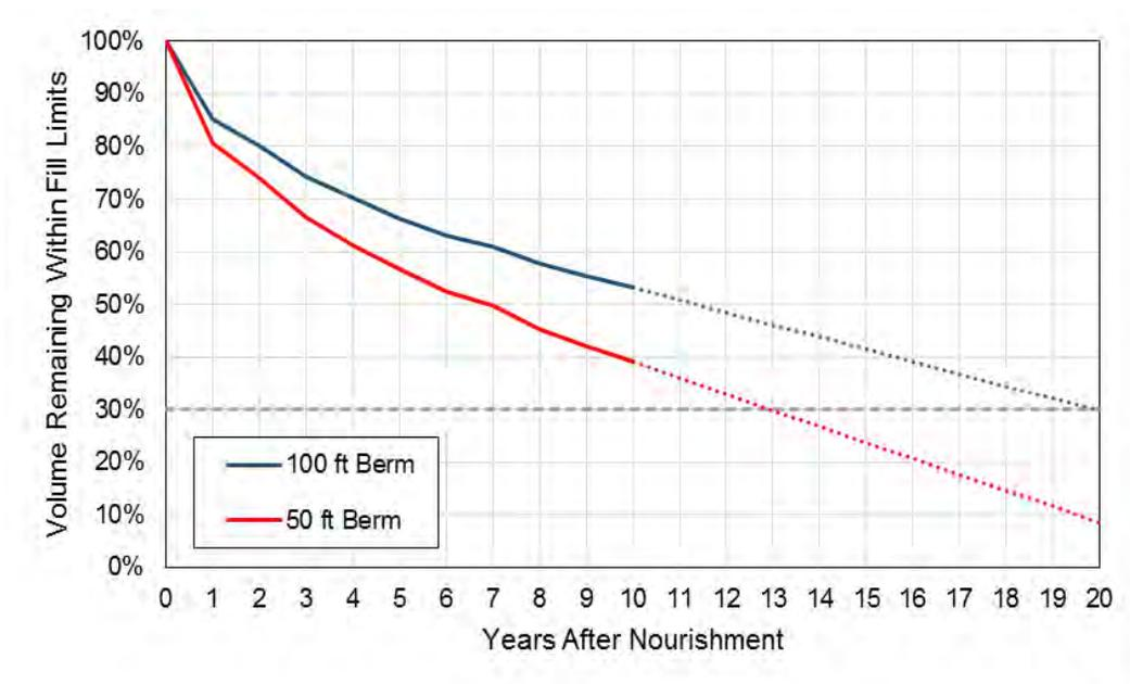
Figure 7.50 Volume of fill remaining over the course of the model simulation for the “long-length” nourishment (Humarock North and South). The dashed gray line indicates the 30% remaining design threshold.
