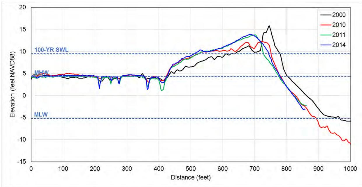
Figure 2.12 Profile change from 2000, 2010, 2011, and 2014 at Transect 3 (Peggotty Beach). In addition to the LiDAR profiles, the dashed lines indicate the elevation of Mean Low Water (MLW), Mean High Water (MHW), and the 100-year Still Water Elevation (100-YR SWL).
