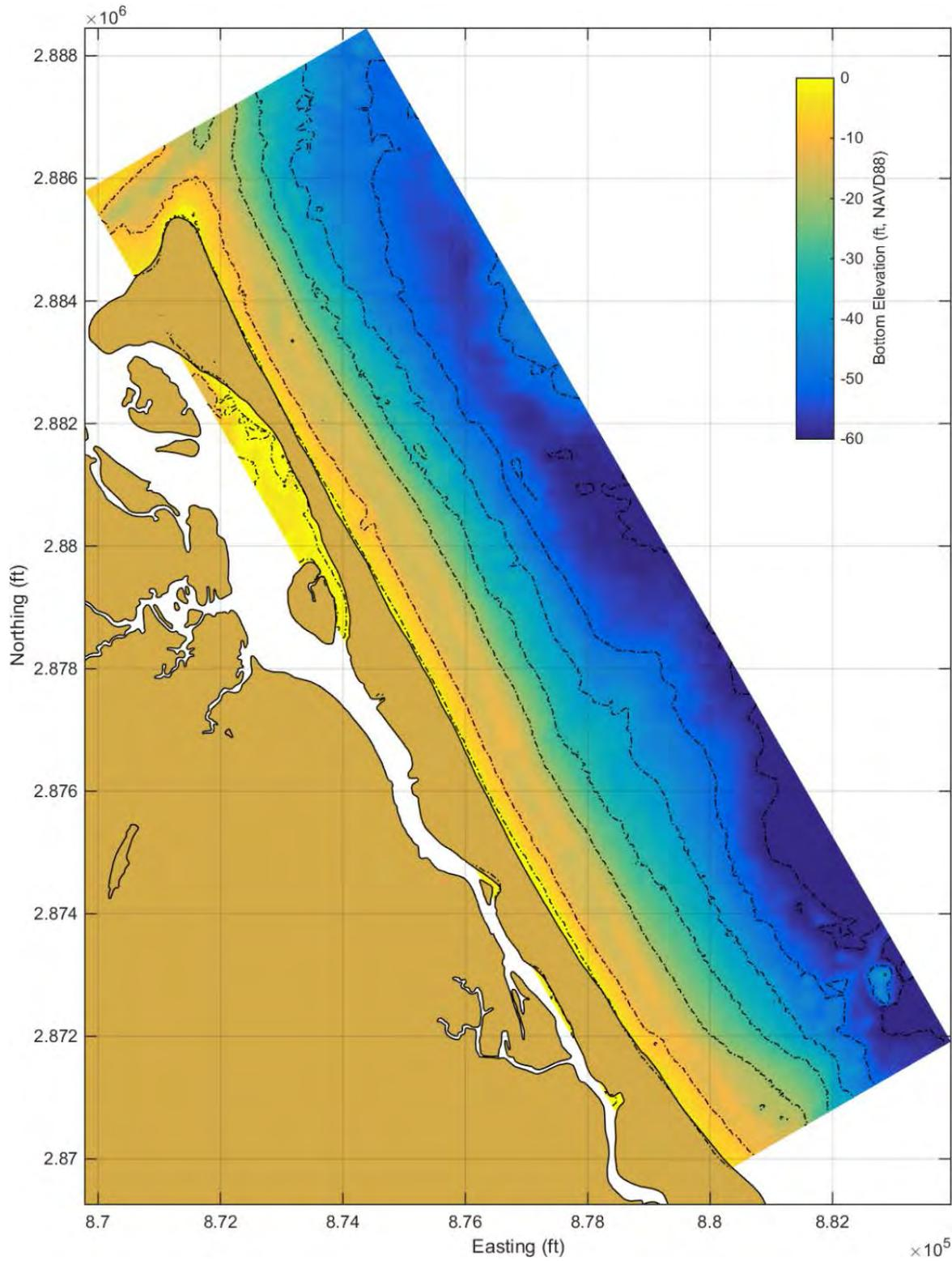
Figure 3.5 Map showing wave model grid limits and bathymetry of the fine model grid of the Scituate shoreline from Fourth Cliff to the southern town limits. 10-foot bathymetric contour lines are also indicated.
