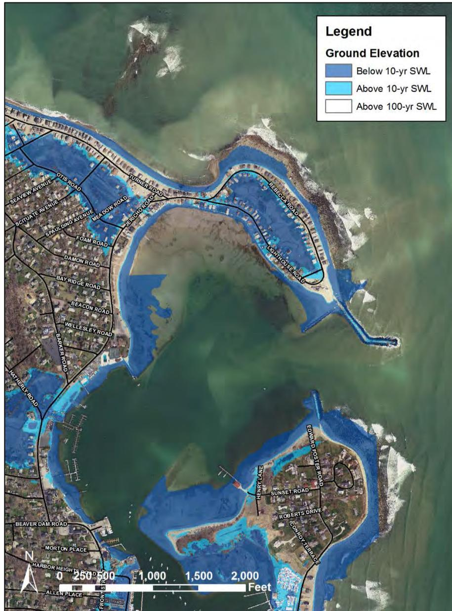
Figure 5.5 Mapping of landform elevation at Cedar Point and First Cliff. Dark and light blue shading indicates that the area is flooded during 10- and 100-year storms by still water (excluding waves), respectively.
