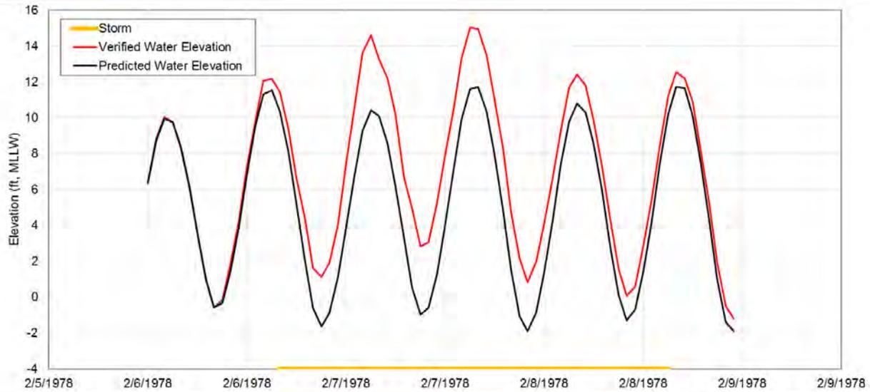
Figure 4.5 Time series plot of the Blizzard of 1978. The black and red lines represent the predicted and observed water elevation, respectively. The yellow line indicates the storm duration.
