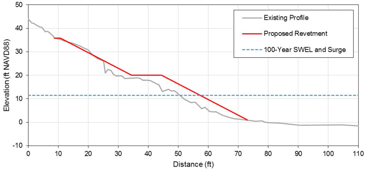
Figure 7.42 Schematic of proposed revetment design along Third Cliff where the revetment is extended to a higher elevation and a berm is added to dissipate wave energy.
