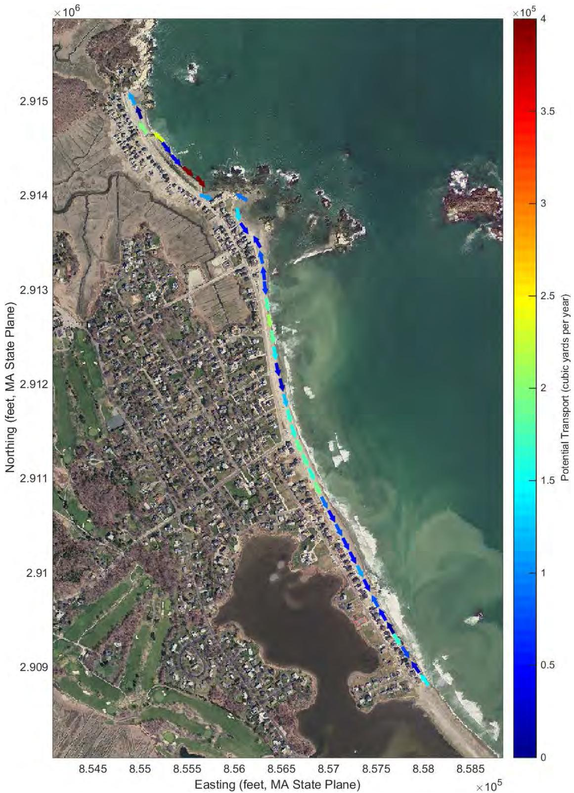
Figure 3.14 Modeled annual potential sediment transport along Minot, North Scituate, and Surfside Beaches. The sediment transport vectors represent the net direction and magnitude of transport along the coast.
