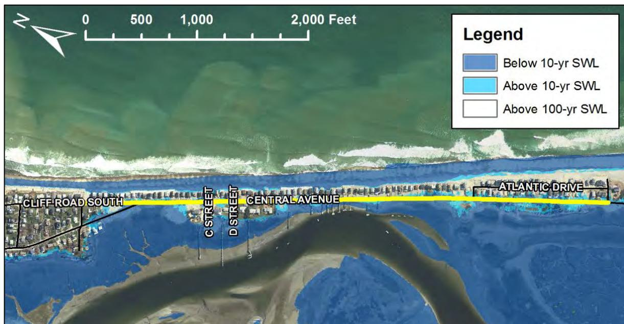
Figure 7.52 Flooding extents of the 10-year and 100-year still water elevation across Central Avenue.
