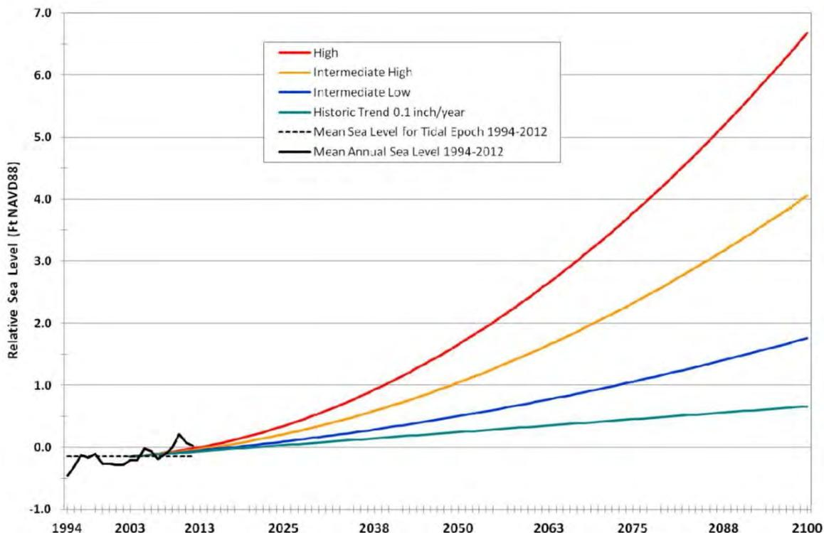
Figure 3.11 Relative sea level rise scenarios estimates (in feet NAVD88) for Boston, MA. Global scenarios from were adjusted to account for local vertical land movement with 2003 as the beginning year of analysis (figure credit: MCZM, 2013).
