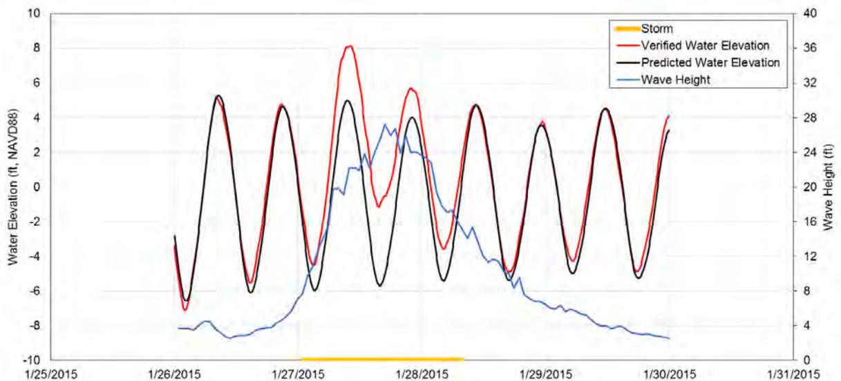
Figure 4.11 Time series plot of Winter Storm Juno. The black and red lines represent the predicted and observed water elevation, respectively. The blue line represents the offshore wave height and the yellow line indicates the storm duration.
