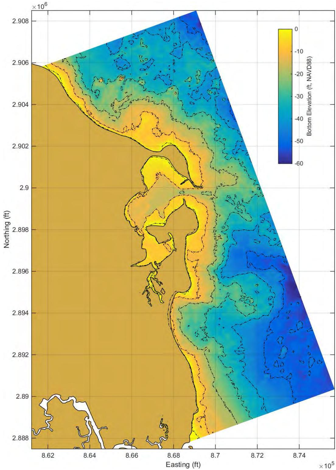
Figure 3.4 Map showing wave model grid limits and bathymetry of the fine model grid of the Scituate shoreline from Egypt Beach to Third Cliff. 10-foot bathymetric contour lines are also indicated.
