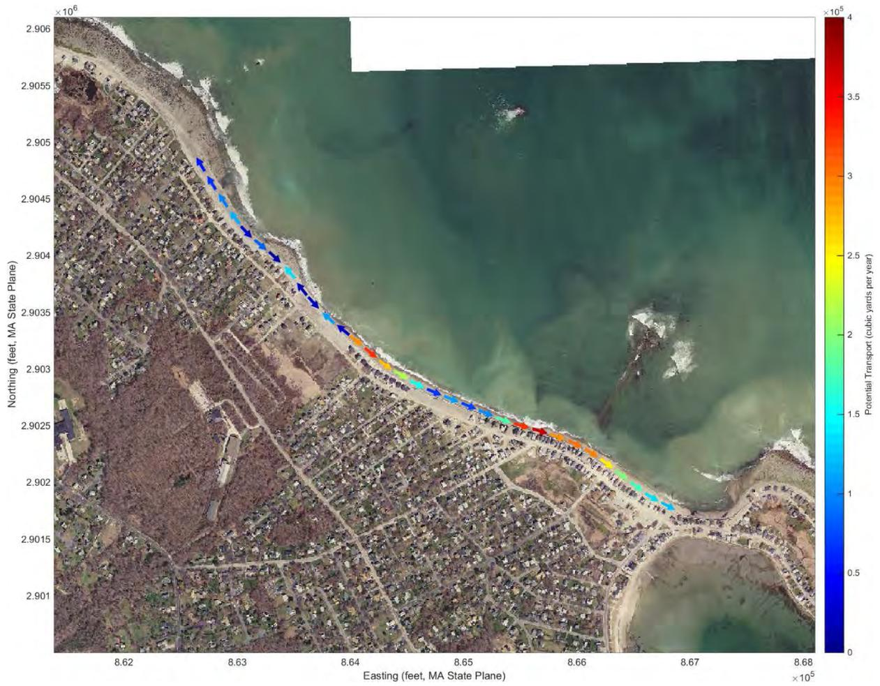
Figure 3.15 Modeled annual potential sediment transport along Oceanside Drive. The sediment transport vectors represent the net direction and magnitude of transport along the coast.
