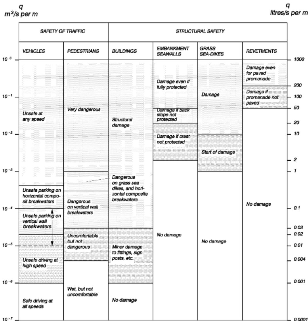
Figure 6.5 Critical values of average overtopping discharges (USACE, 2002).
