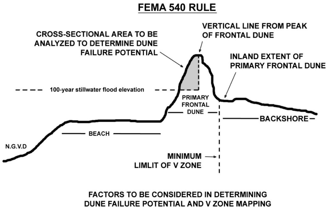
Figure 6.9 FEMA 540 Rule for determining dune failure potential (image credit: FEMA).
