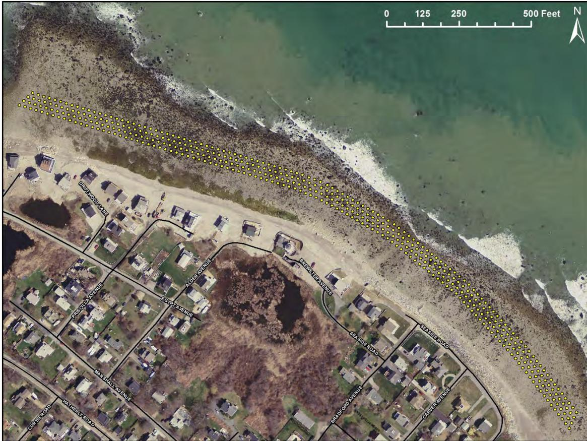
Figure 7.17 Configuration of individual boulders (represented by the yellow circles) forming a boulder dike along Egypt Beach from Bay Street to Standish Avenue.
