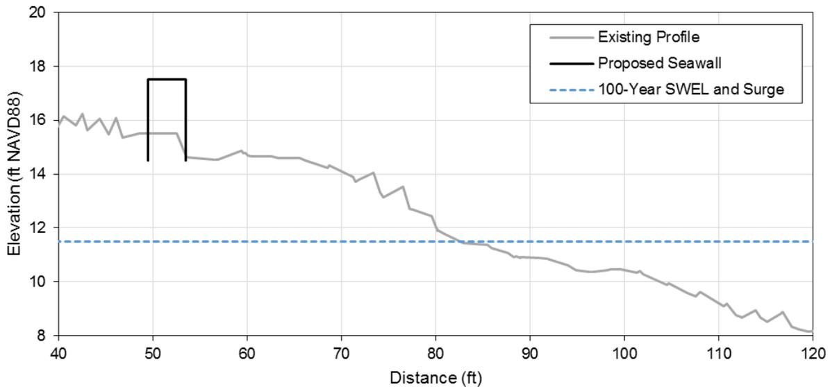
Figure 7.55 Schematic of the proposed design along Humarock South where the seawall height is increased by 2 feet.
