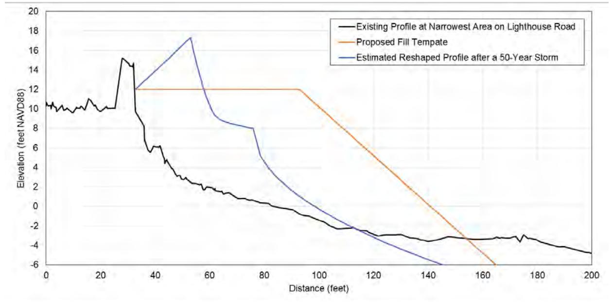
Figure 7.24 Existing profile, proposed fill template, and reshaped profile after a 50-year storm at the narrowest area on Lighthouse Road.
