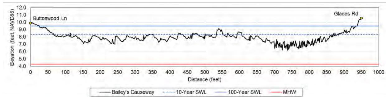
Figure 7.7 Road elevation along Bailey’s Causeway from Buttonwood Lane to Glades Road.
