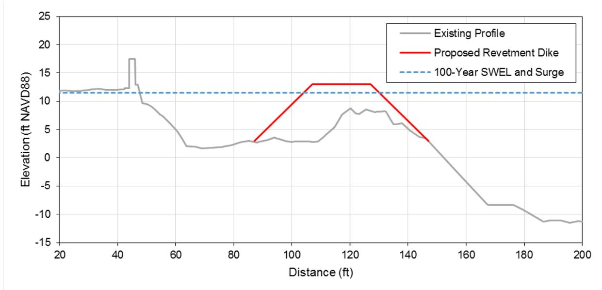
Figure 7.4 Schematic of proposed revetment dike design along Minot Beach where the crest of the existing revetment dike is raised and widened and the seawall is unaltered.
