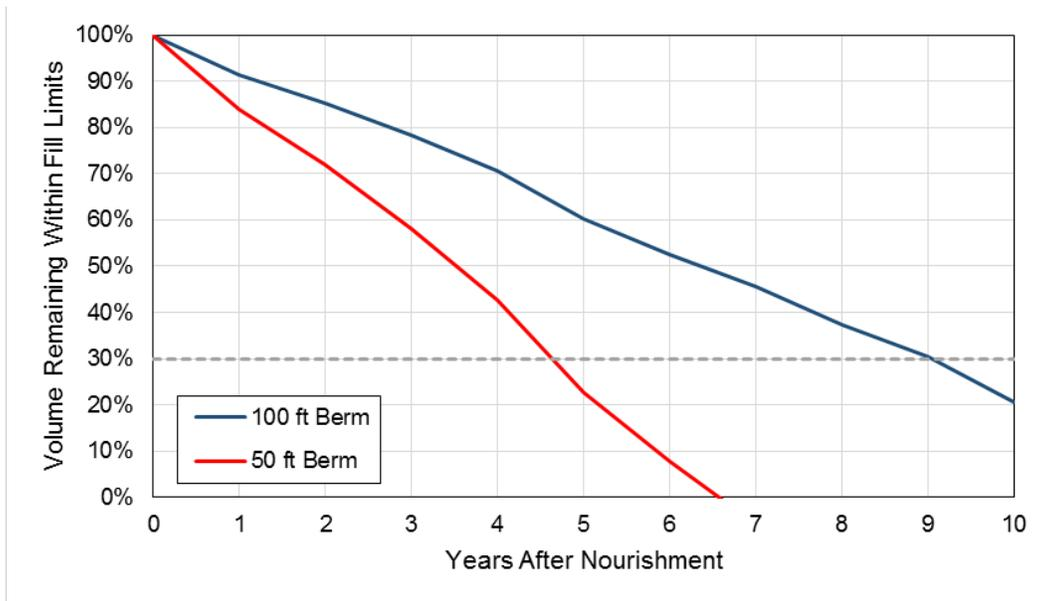
Figure 7.37 Volume of fill remaining over the course of the model simulation for a nourishment along the entire length of Peggotty Beach. The dashed gray line indicates the 30% remaining design threshold.
