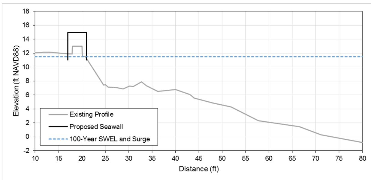
Figure 7.1 Schematic of the proposed seawall design along Minot Beach (north wall section) where the seawall height is increased by 2 feet.
