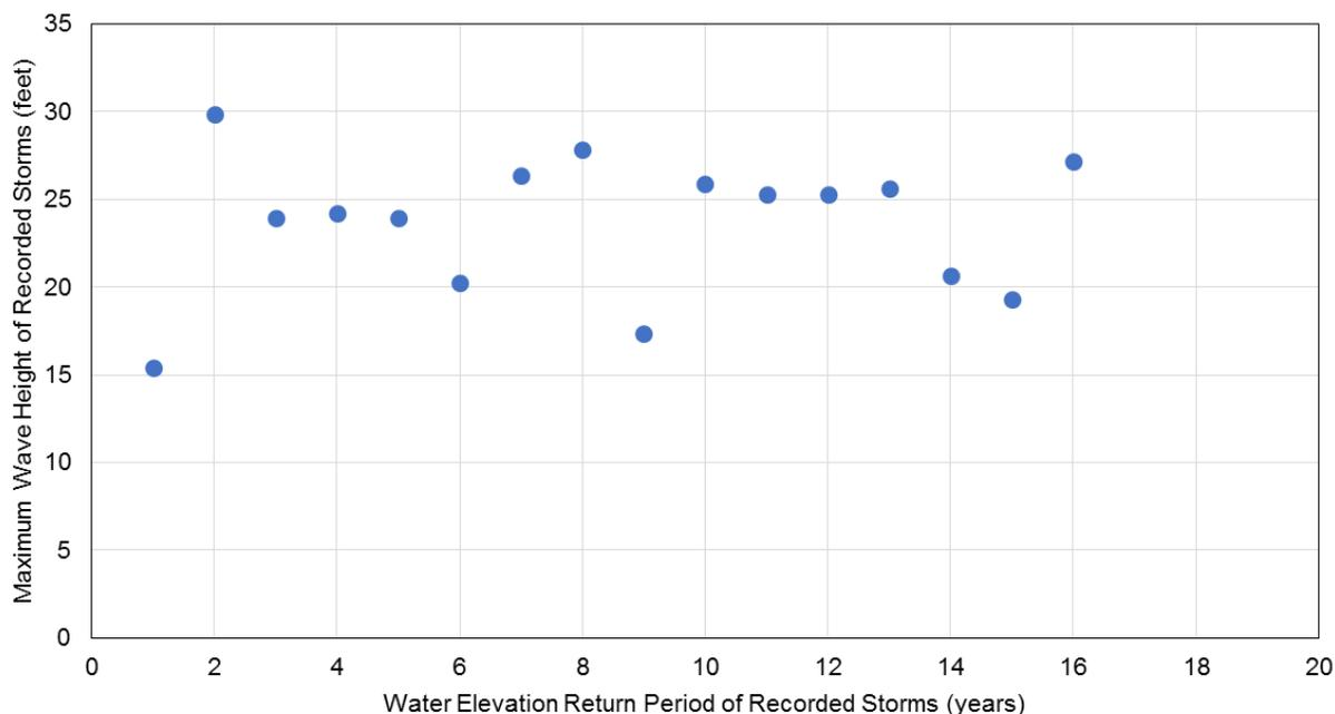
Figure 4.4 Recorded maximum wave height at National Data Buoy Center Station 44013 versus maximum storm surge elevations recorded for a range of storm return periods based upon tide level observations at NOAA Station 8443970.
