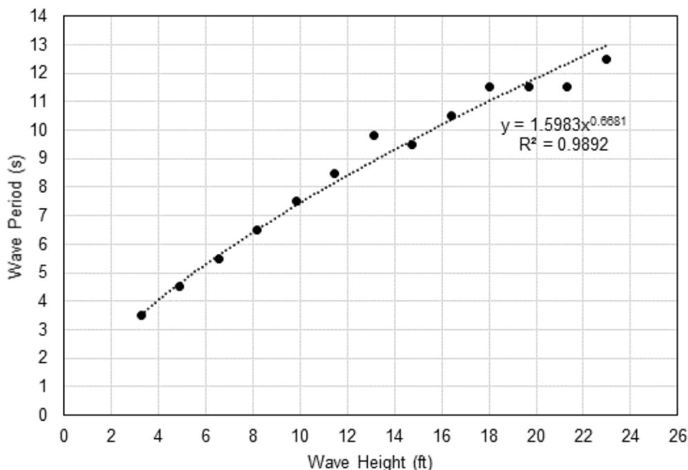
Figure 3.9 Wave period and wave height relationship for WIS hindcast station 63053.
