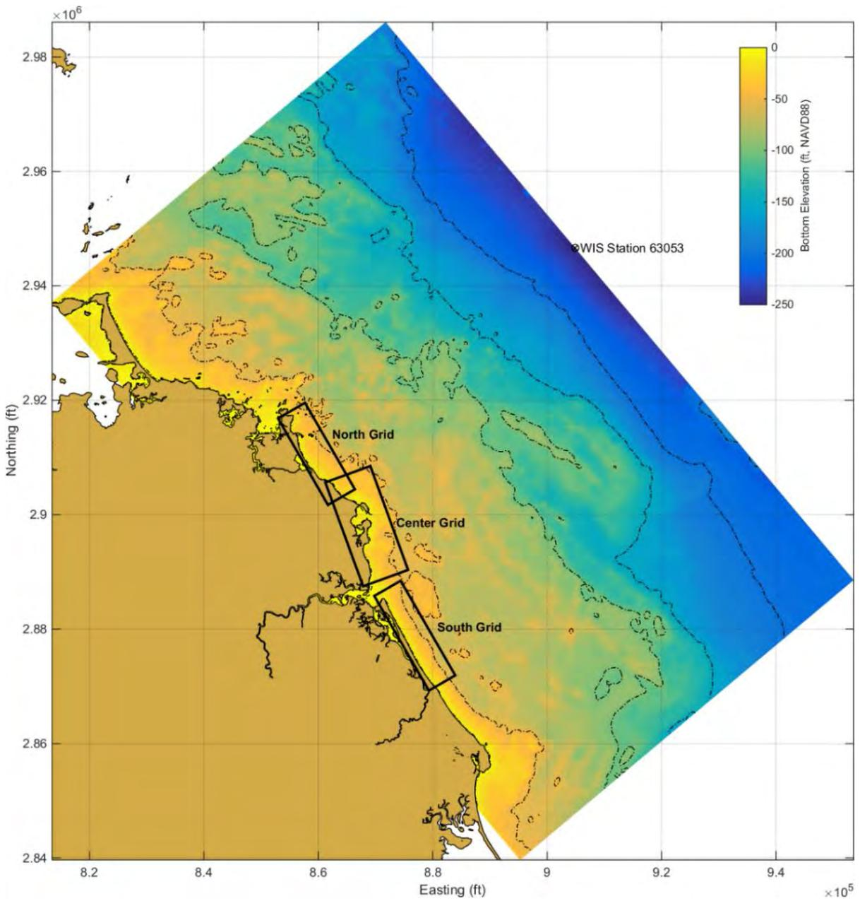
Figure 3.2 Map showing wave model grid limits and bathymetry of both the coarse model grid the offshore area between the WIS wave station and the Massachusetts coast. 50-foot bathymetric contour lines are also shown.
