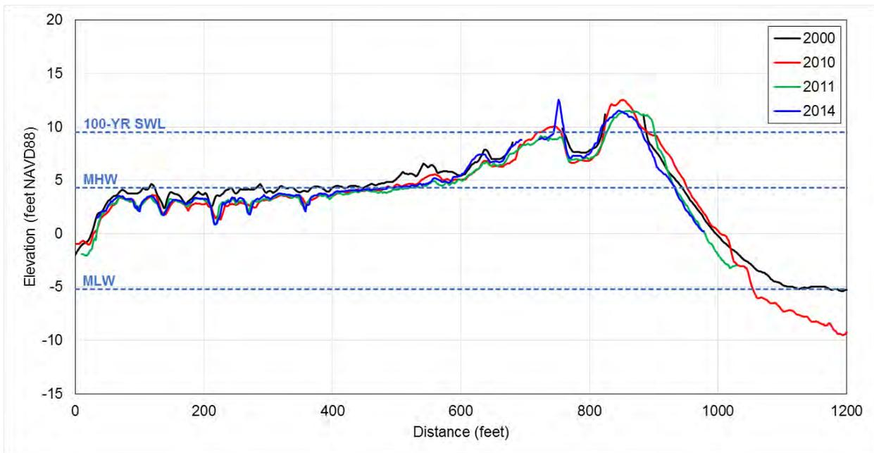
Figure 2.14 Profile change from 2000, 2010, 2011, and 2014 at Transect 4 (north section of Humarock Beach). In addition to the LiDAR profiles, the dashed lines indicate the elevation of Mean Low Water (MLW), Mean High Water (MHW), and the 100-year Still Water Elevation (100-YR SWL).
