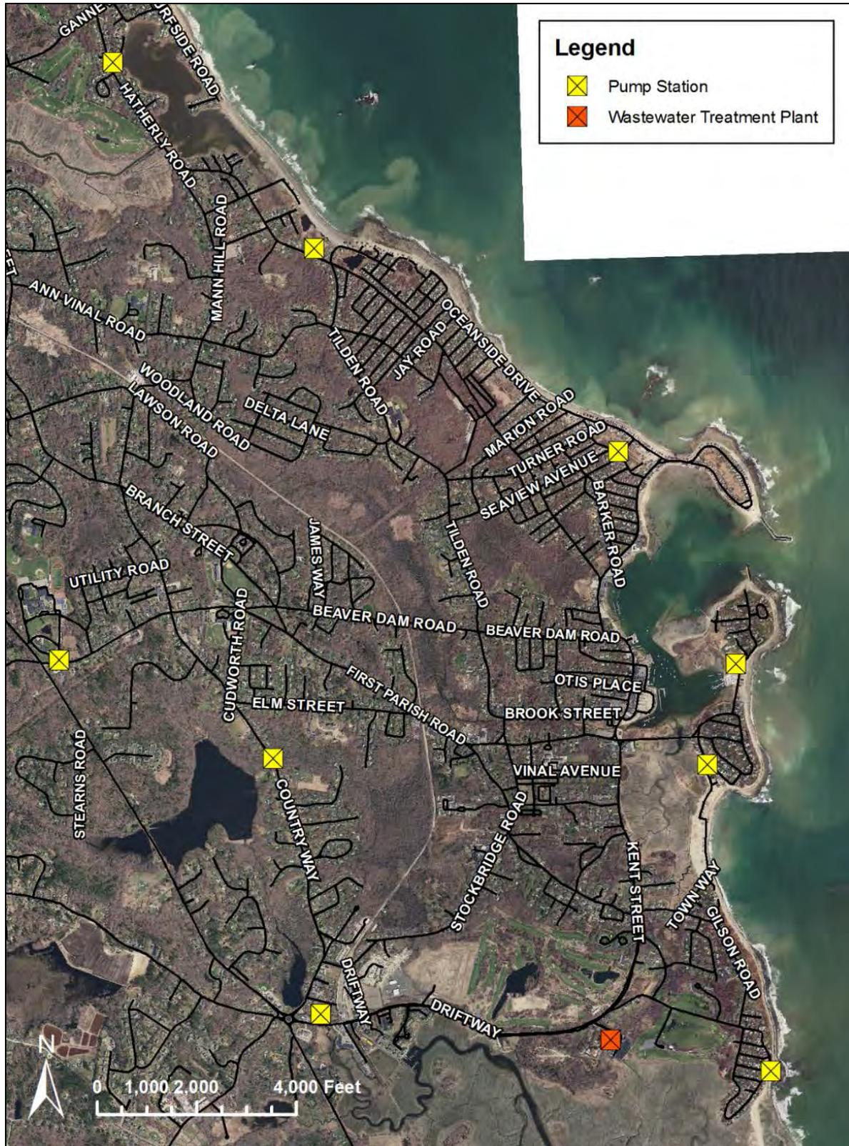
Figure 5.8 Pump stations and wastewater treatment plant in Scituate.
