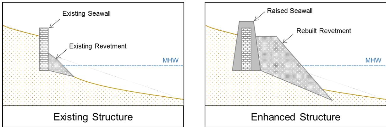
Figure 6.3 Schematic of the existing seawall and revetment structure (left) and the enhanced structure (right) which involves raising the seawall and a larger fronting revetment to dissipate wave energy and reduce overtopping.
