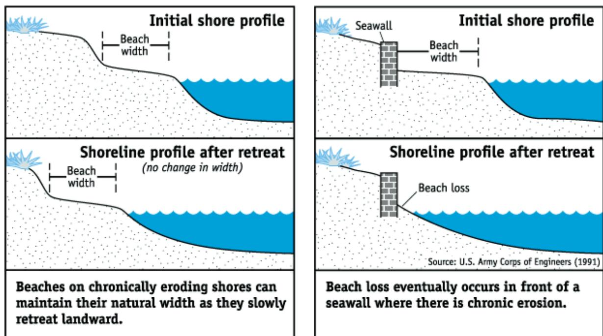
Figure 6.1 Chronic beach erosion on unhardened shores (left) and with seawalls in place (right) (image credit: U.S. Army Corps of Engineers).
