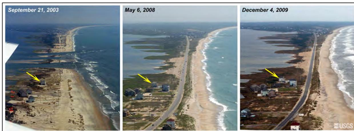
Figure 5.10 Oblique aerial photography looking north along Hatteras Island, NC on September 21, 2003 (left, after hurricane Isabel), May 6, 2008 (middle) and December 4, 2009 (right), roughly two weeks after the storm. The yellow arrows point to the same location in each photograph. The inlet formed during Isabel was filled, and a protective dune was constructed in front of the new road (*image credit: USGS*).
