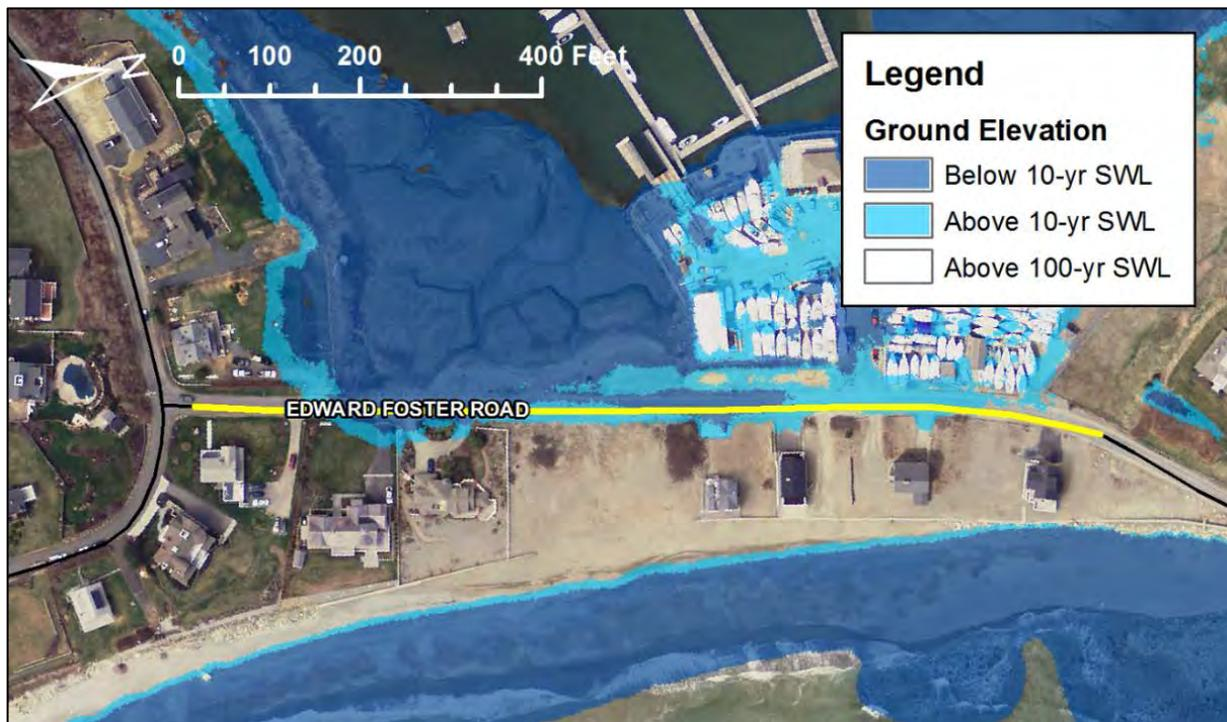
Figure 7.28 Flooding extents of the 10-year and 100-year still water elevation across Edward Foster Road.
