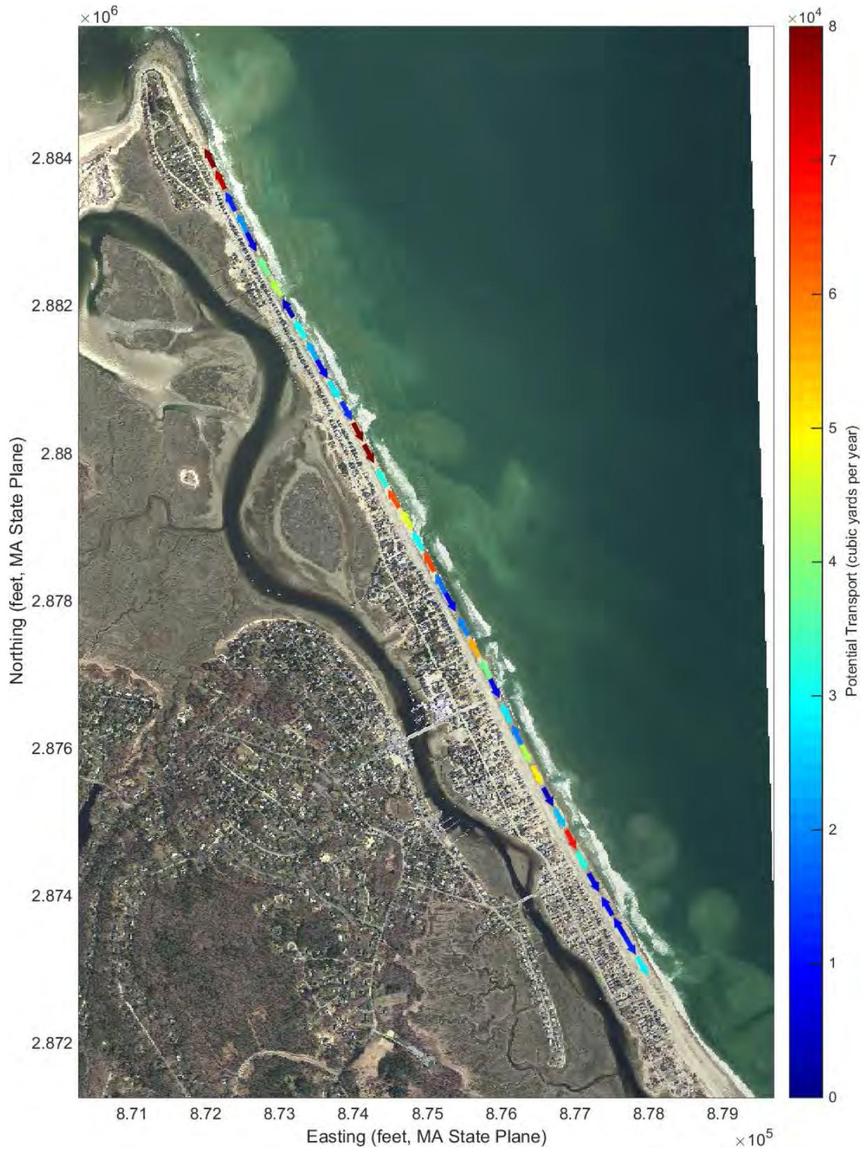
Figure 3.16 Modeled annual potential sediment transport along Humarock Beach. The sediment transport vectors represent the net direction and magnitude of transport along the coast.
