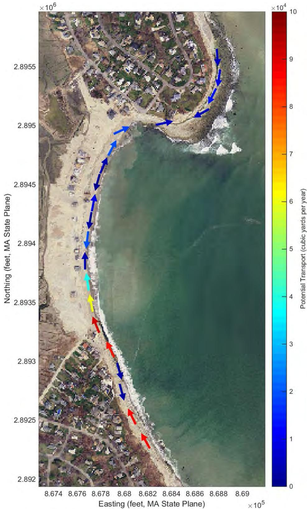
Figure 3.13 Modeled annual potential sediment transport at Peggotty Beach. The sediment transport vectors represent the net direction and magnitude of transport along the coast.
