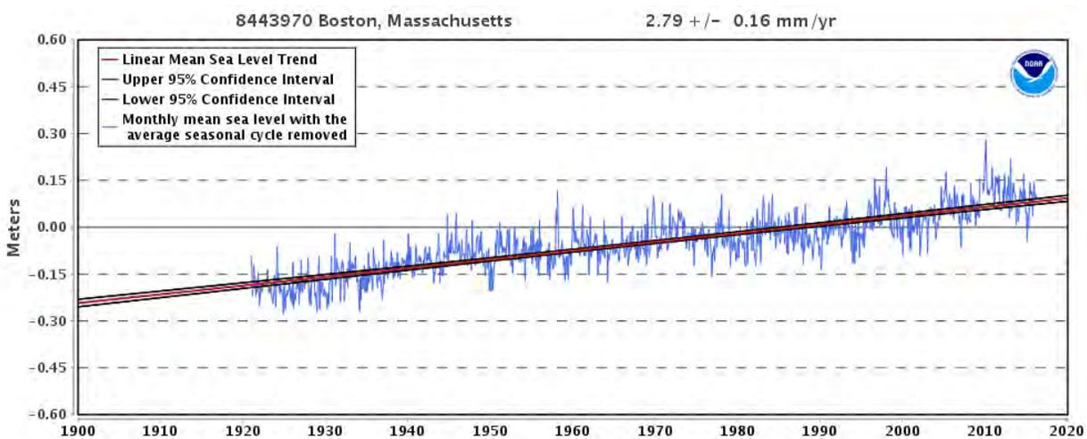
Figure 3.10 Long-term mean sea level data for NOAA Boston tide gauge station with linear trend and confidence interval.
