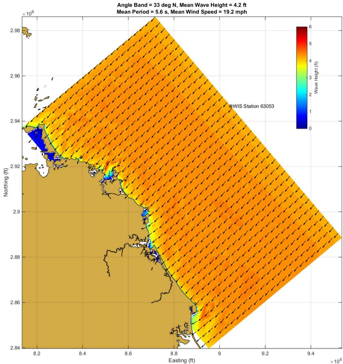
Figure 3.6 Coarse grid output for case 4 (angle band = 33 deg, mean wave height = 4.1 ft, mean wave period = 5.6 s, mean wind speed = 19.2 mph). Color contours indicate wave heights and vectors show peak wave direction.
