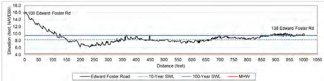
Figure 7.29 Road elevation from 100 Edward Foster Road to 138 Edward Foster Road.
