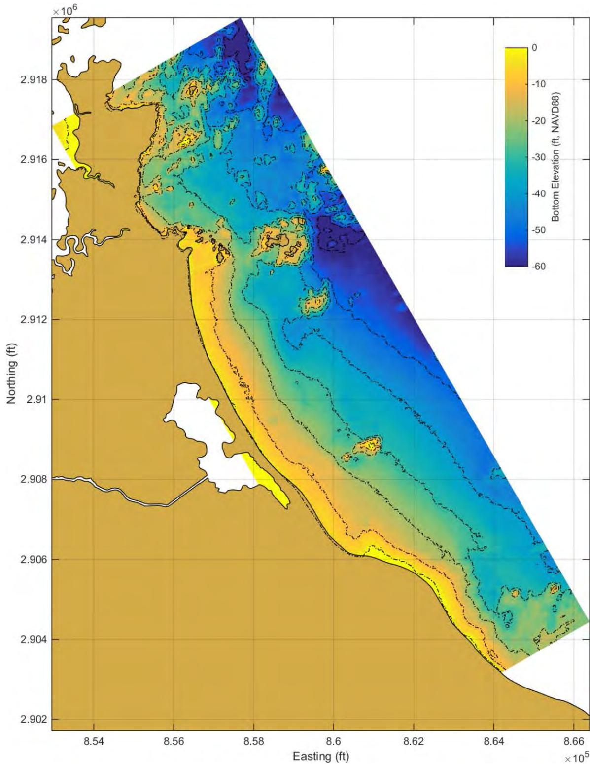
Figure 3.3 Map showing wave model grid limits and bathymetry of the fine model grid of the Scituate shoreline from Scituate Neck to Egypt Beach. 10-foot bathymetric contour lines are also indicated.
