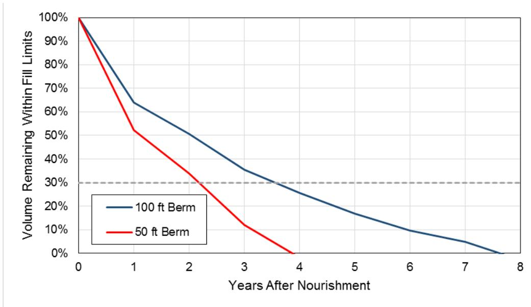
Figure 7.49 Volume of fill remaining over the course of the model simulation for the “short-length” nourishment (Humarock North only). The dashed gray line indicates the 30% remaining design threshold.
