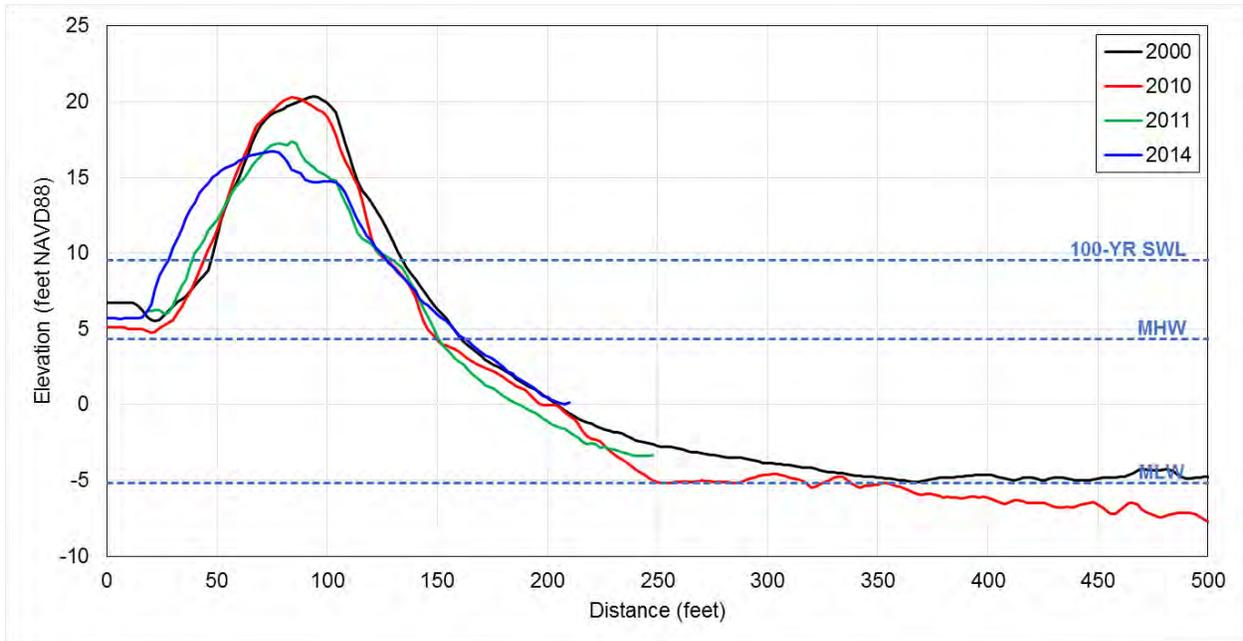
Figure 2.10 Profile change from 2000, 2010, 2011, and 2014 at Transect 2 (Egypt Beach). In addition to the LiDAR profiles, the dashed lines indicate the elevation of Mean Low Water (MLW), Mean High Water (MHW), and the 100-year Still Water Elevation (100-YR SWL).
