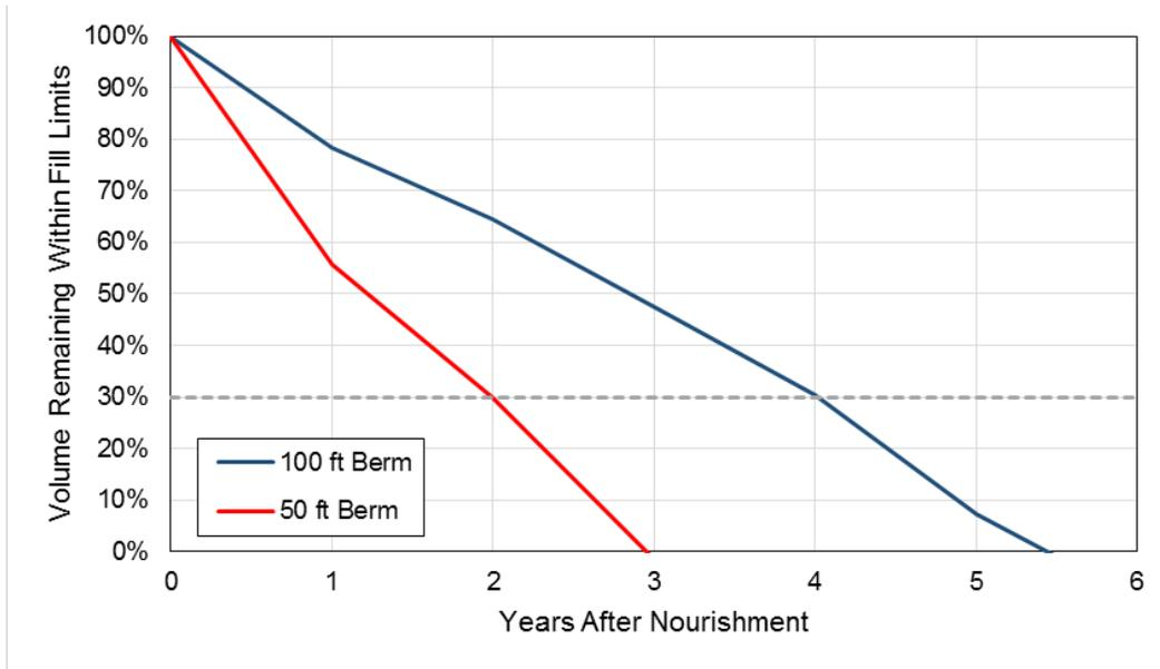
Figure 7.36 Volume of fill remaining over the course of the model simulation for a nourishment along the northern area of Peggotty Beach. The dashed gray line indicates the 30% remaining design threshold.
