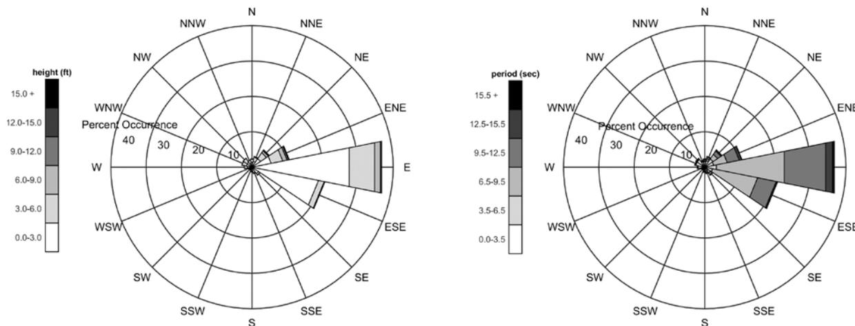
Figure 3.1 Wave height and period for hindcast data from WIS station 63053 (11 miles offshore Scituate Neck) for the 33-year period between January 1980 and December 2012. Direction indicates from where waves were traveling, relative to true north. Radial length of gray tone segments indicates percent occurrence for each range of wave heights and periods. Combined length of segments in each sector indicate percent occurrence of all waves from that direction.
