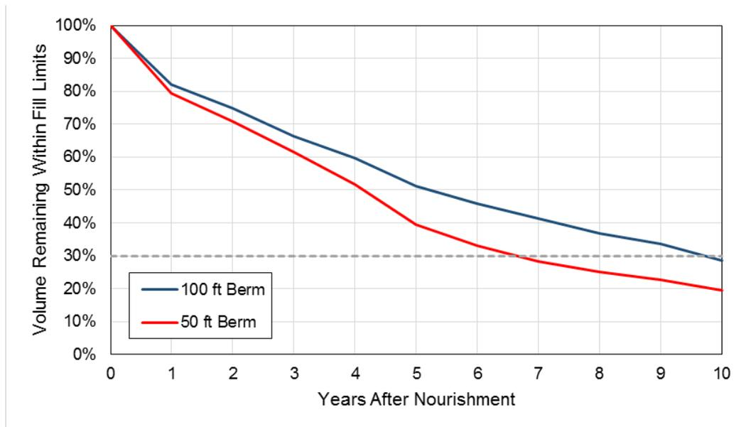
Figure 7.20 Volume of fill remaining over the course of the model simulation for two nourishment options along Oceanside Drive. The dashed gray line indicates the 30% remaining design threshold.
