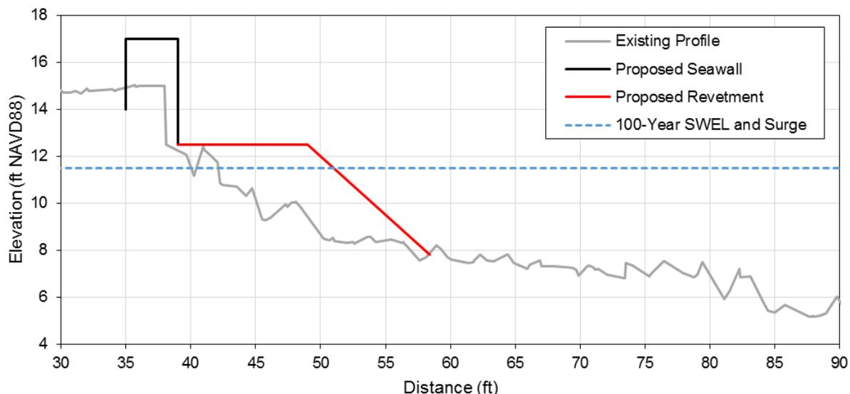
Figure 7.46 Schematic of the proposed seawall and revetment design along Humarock North where the seawall height is increased by 2 feet and the fronting revetment is expanded.
