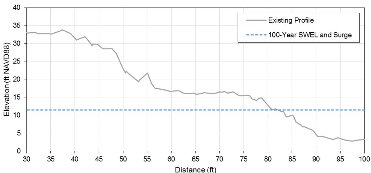
Figure 7.26 Profile of the existing revetment along First Cliff.
