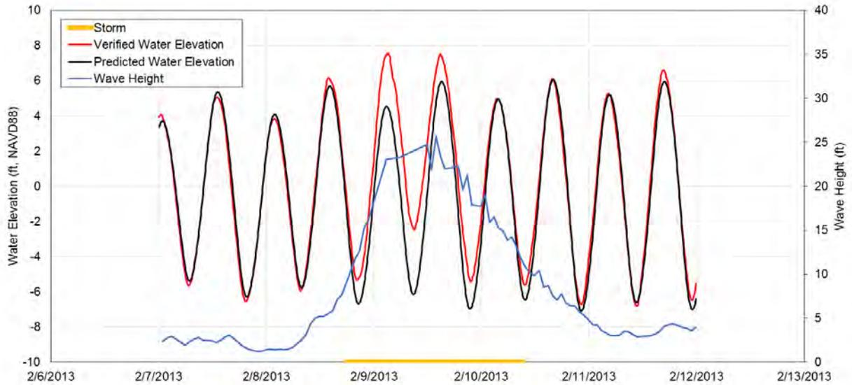
Figure 4.10 Time series plot of Winter Storm Nemo. The black and red lines represent the predicted and observed water elevation, respectively. The blue line represents the offshore wave height and the yellow line indicates the storm duration.
