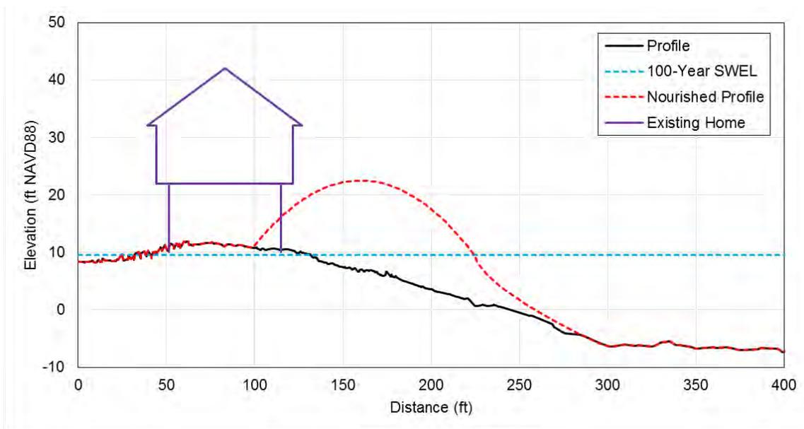
Figure 7.51 Schematic of the proposed dune profile required to satisfy the “540 rule” along Humarock North.
