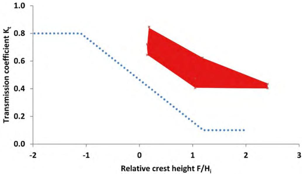
Figure 6.20 Figure from Douglass et al. (2012) showing the wave transmission coefficients of the laboratory experiments for a breakwater consisting of 4-sided apex-truncated square pyramid shaped breakwater units (red data envelope show) compared to coefficients of a traditional stone breakwater in blue.
