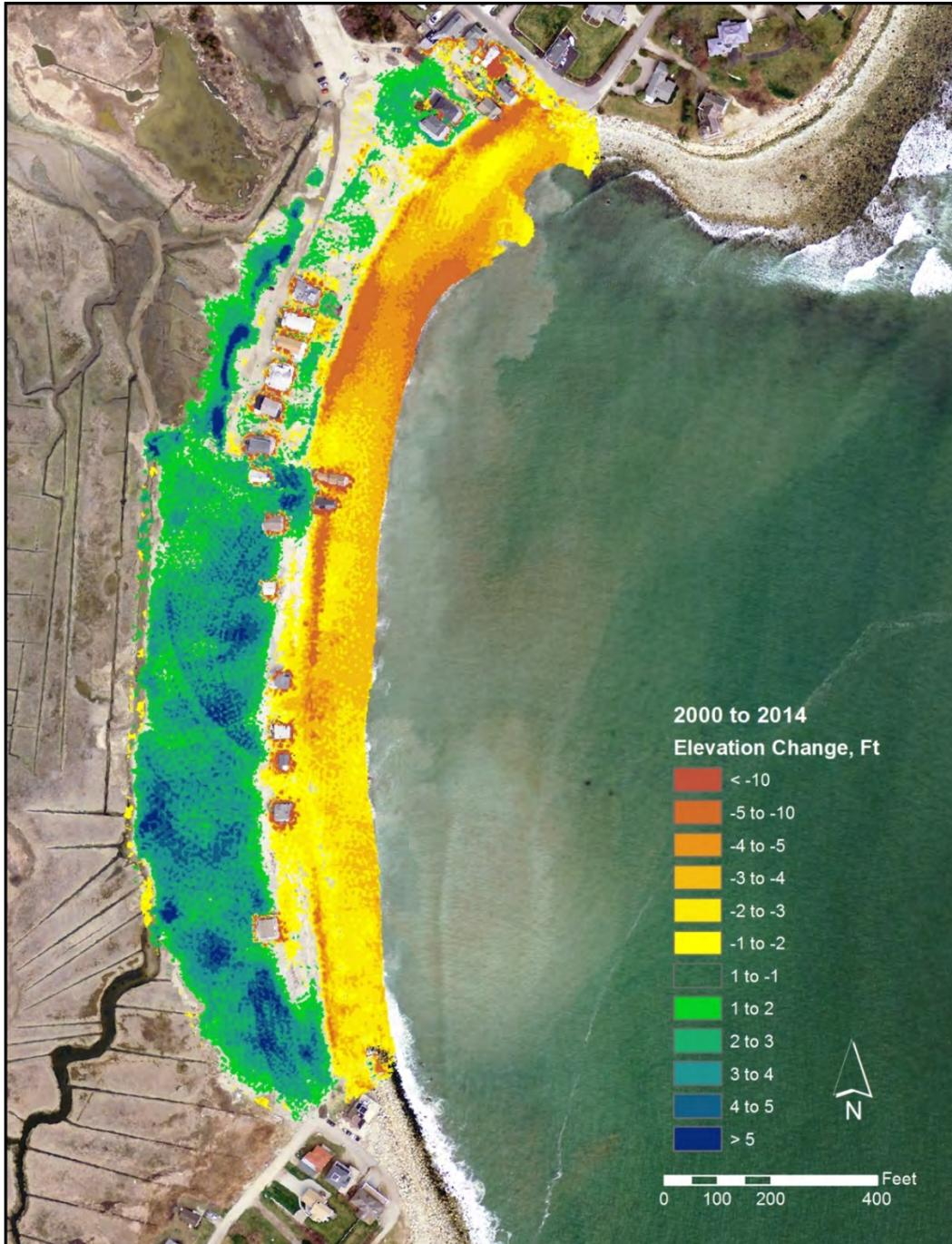
Figure 2.18 Topographic change from LiDAR data computed between 2000 and 2014 for Peggotty Beach, where negative values indicate erosion and positive values indicate accretion.
