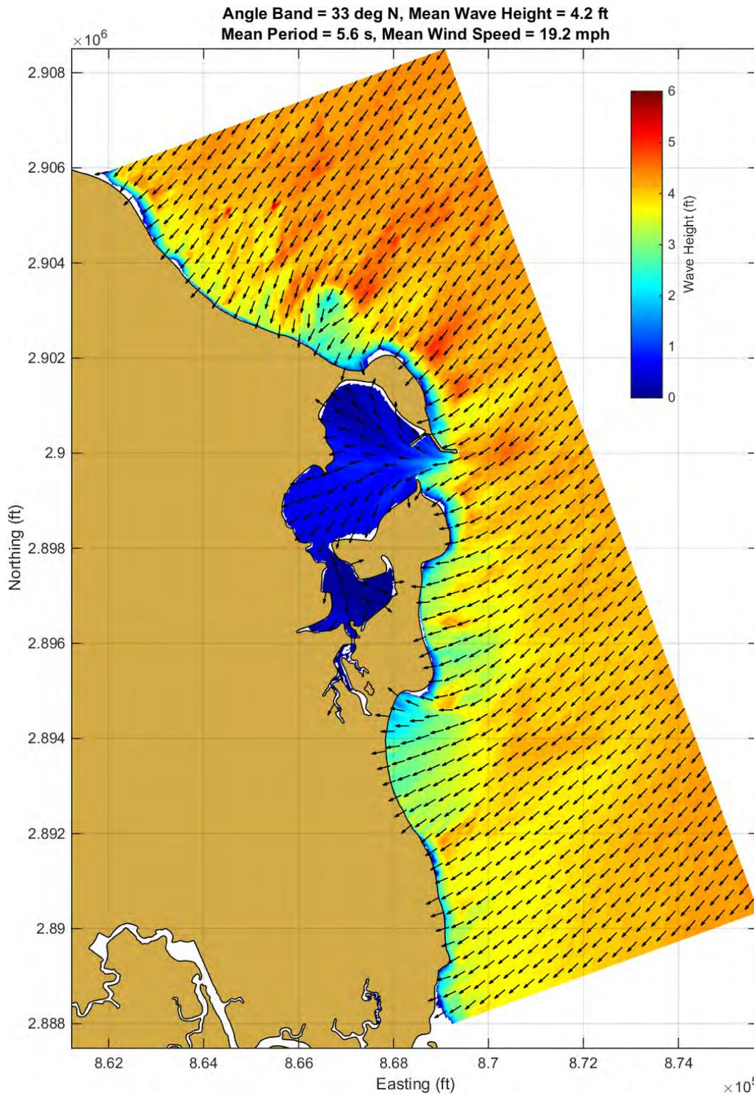
Figure 3.7 Fine grid output for case 4 (angle band = 33 deg, mean wave height = 4.1 ft, mean wave period = 5.6 s, mean wind speed = 19.2 mph). Color contours indicate wave heights and vectors show peak wave direction.
