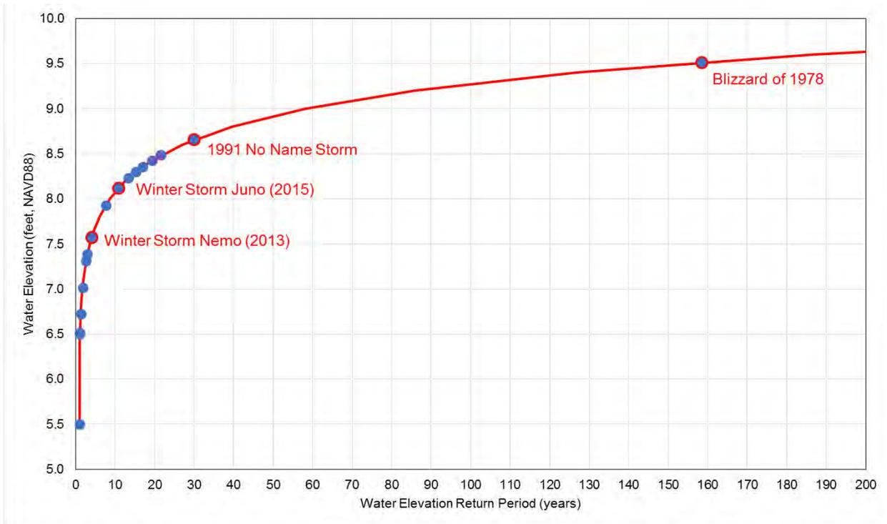
Figure 4.1 Water elevation return period of selected storm. Water elevations are measured in Boston at NOAA Station 8443970.
