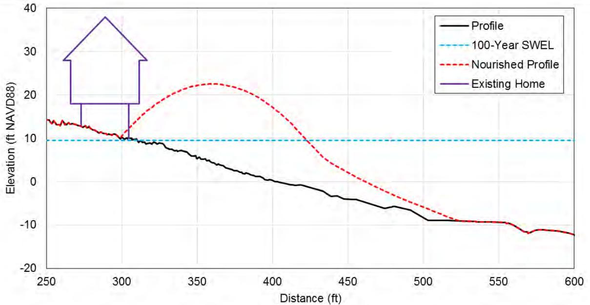
Figure 7.40 Schematic of the dune profile required to satisfy the “540 rule” along the southern portion of Peggotty Beach.
