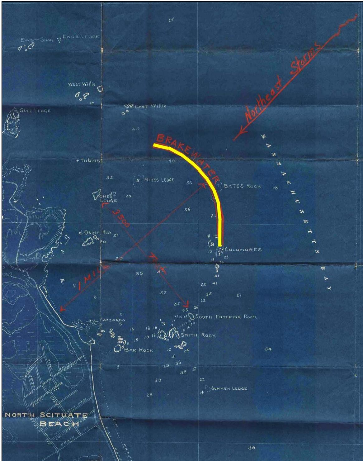
Figure 6.10 Offshore breakwater concept for the Minot Beach area, where the approximate 3,500 feet breakwater would serve to protect about ½ mile of beach (Source: 1911 Plan from Fred Tupper, C.E.).
