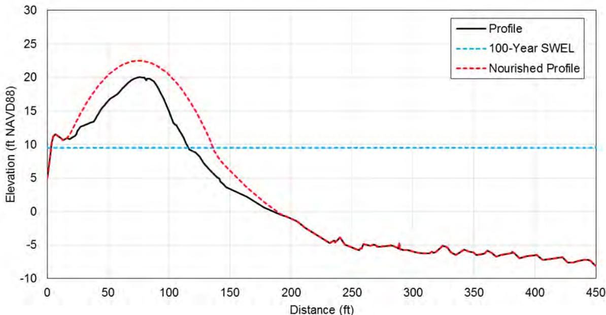
Figure 7.15 Schematic of the dune profile required to satisfy the “540 rule” along Egypt Beach.
