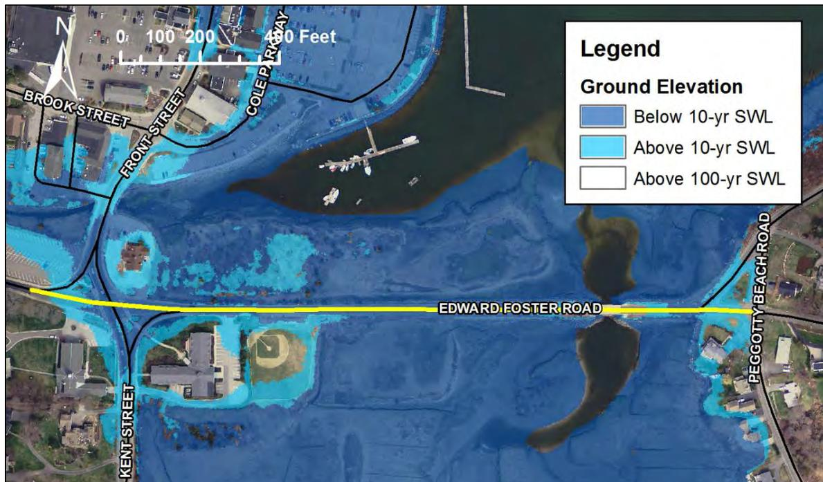
Figure 7.30 Flooding extents of the 10-year and 100-year still water elevation across Edward Foster Road (causeway).
