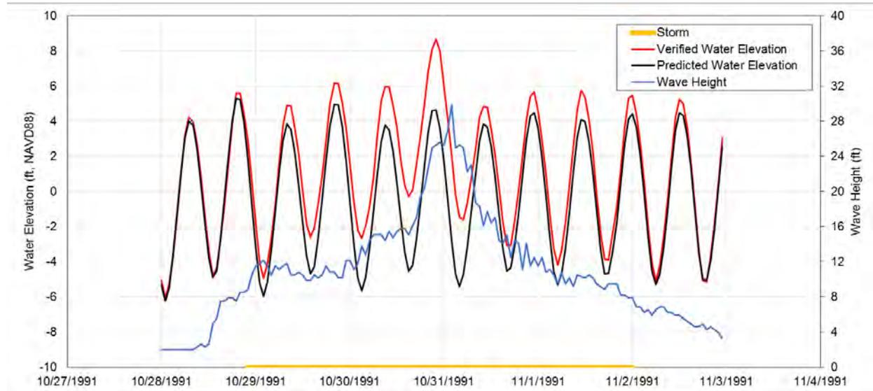
Figure 4.7 Time series plot of the 1991 No-Name Storm. The black and red lines represent the predicted and observed water elevation, respectively. The blue line represents the offshore wave height and the yellow line indicates the storm duration.
