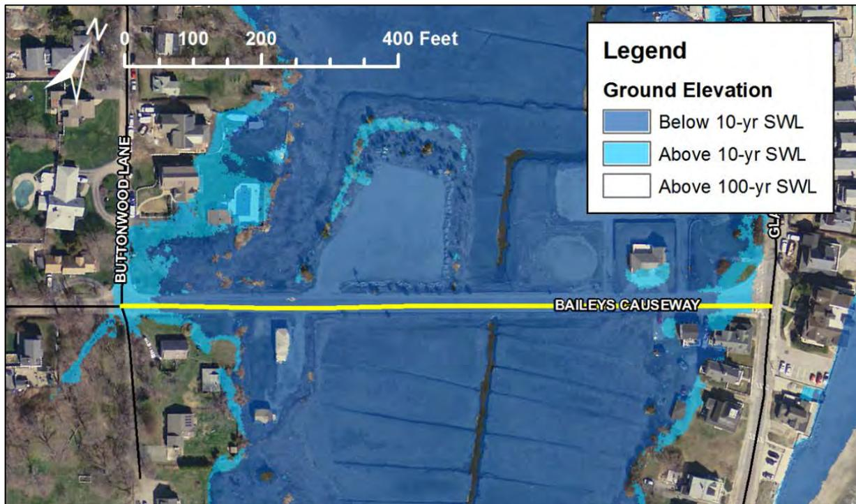
Figure 7.6 Flooding extents of the 10-year and 100-year still water elevation across Bailey’s Causeway.
