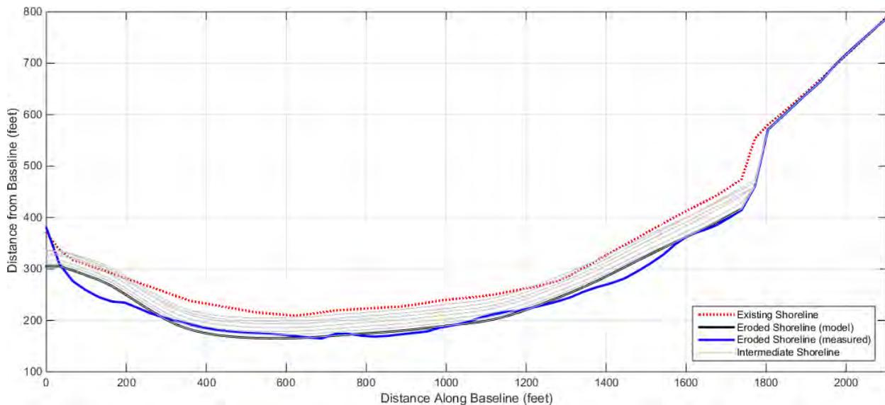
Figure 3.12 Comparison of measured and modeled shorelines along Peggotty Beach.
