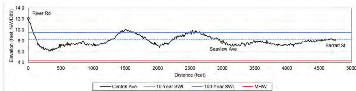
Figure 7.53 Road elevation along Central Avenue from River Road to Barratt Street.
