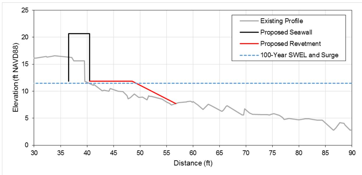
Figure 7.27 Schematic of the proposed seawall and revetment design along Edward Foster Road where the seawall height is increased by 4.7 feet and the fronting revetment is expanded.
