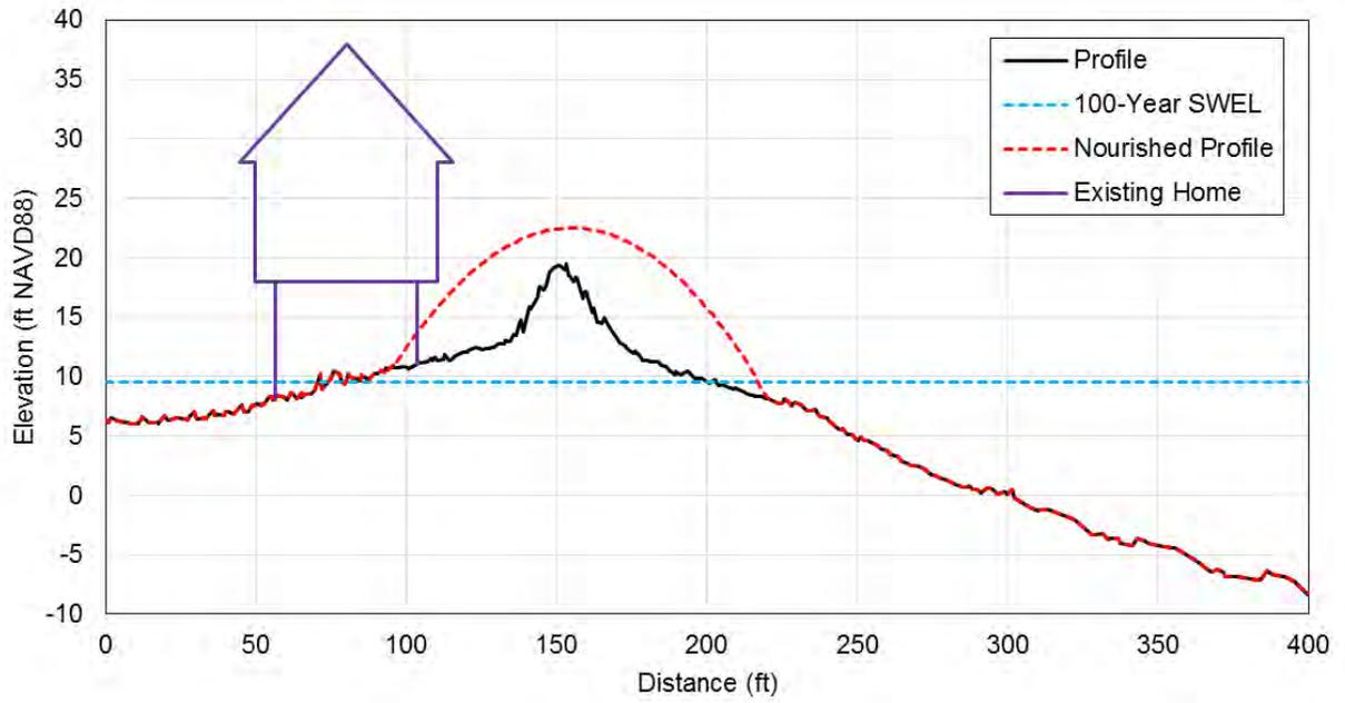
Figure 7.39 Schematic of the proposed dune profile required to satisfy the “540 rule” along the northern portion of Peggotty Beach.
