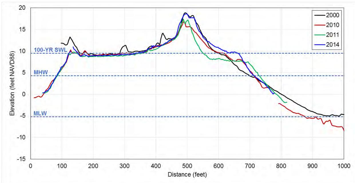
Figure 2.16 Profile change from 2000, 2010, 2011, and 2014 at Transect 5 (south section of Humarock Beach). In addition to the LiDAR profiles, the dashed lines indicate the elevation of Mean Low Water (MLW), Mean High Water (MHW), and the 100-year Still Water Elevation (100-YR SWL).
