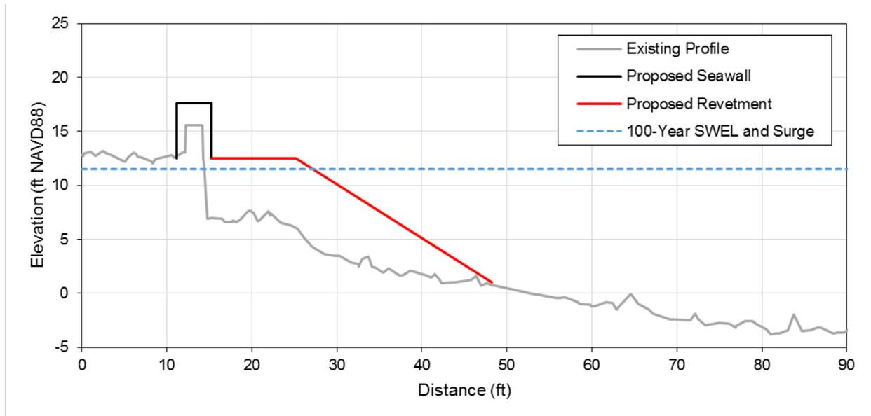
Figure 7.21 Schematic of proposed seawall and revetment design along Cedar Point (Rebecca Road) where the seawall height is increased by 2 feet and the fronting revetment is expanded.
