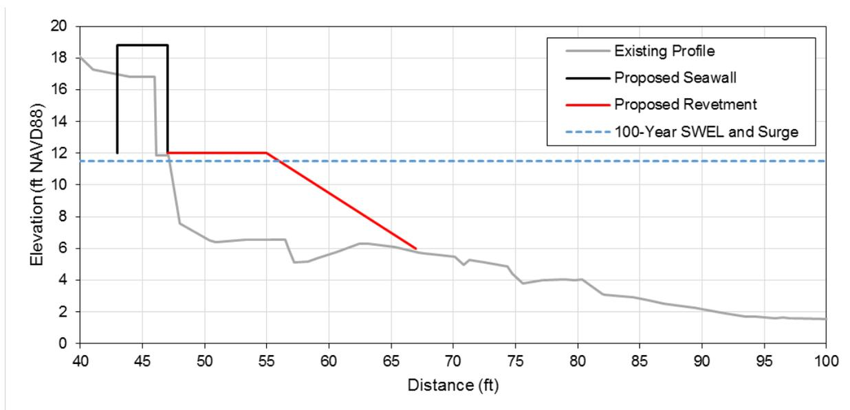
Figure 7.9 Schematic of proposed seawall and revetment design along North Scituate Beach where the seawall height is increased by 2 feet and the fronting revetment is expanded.
