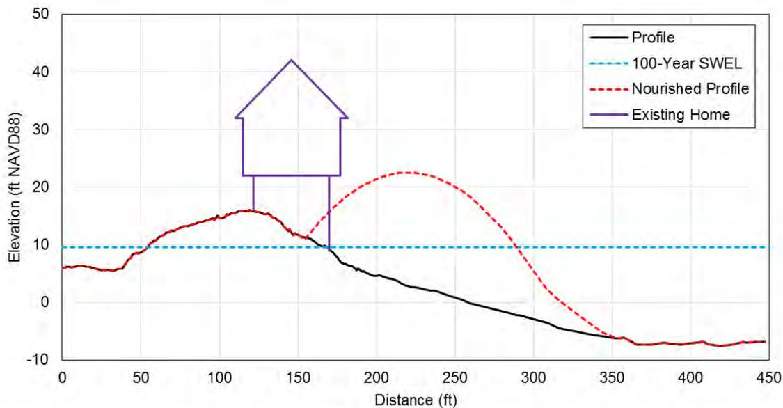
Figure 7.14 Schematic of the dune profile required to satisfy the “540 rule” along Mann Hill Beach.
