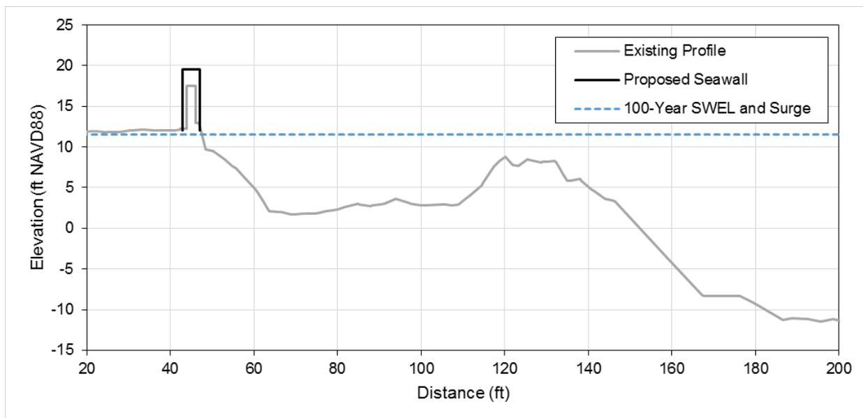
Figure 7.2 Schematic of the proposed seawall design along Minot Beach (south wall section) where the seawall height is increased by 2 feet.
