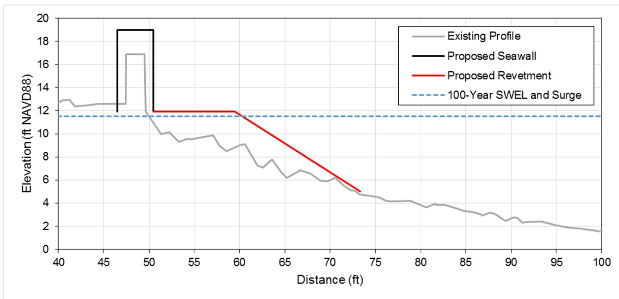
Figure 7.18 Schematic of proposed design along Oceanside Drive where the seawall height is increased by 2 feet and the fronting revetment is expanded.
