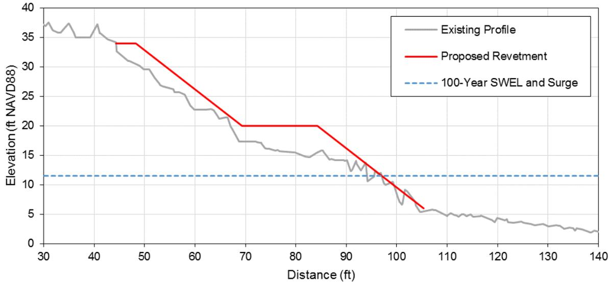
Figure 7.45 Schematic of proposed design along Fourth Cliff where the revetment is extended to a higher elevation and a berm is added to dissipate wave energy.
