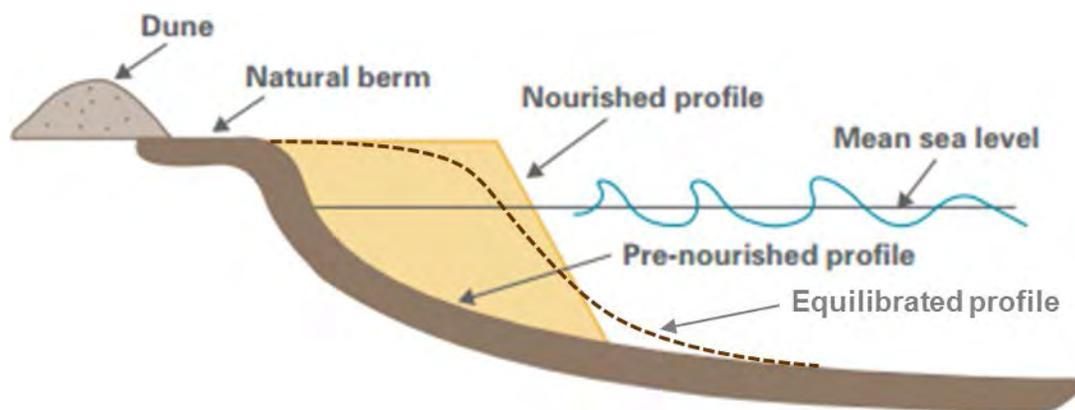
Figure 6.7 Cross-sectional schematic of a beach profiles before nourishment, immediate after nourishment, and after equilibration (*image credit: American Shore and Beach Preservation Association - modified*).
