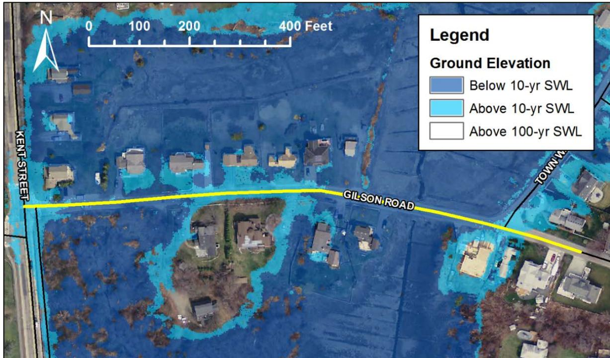
Figure 7.43 Flooding extents of the 10-year and 100-year still water elevation across Gilson Road.
