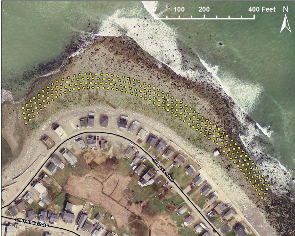
Figure 7.25 Configuration of individual boulders (represented by the yellow circles) forming a boulder dike along Cedar Point.
