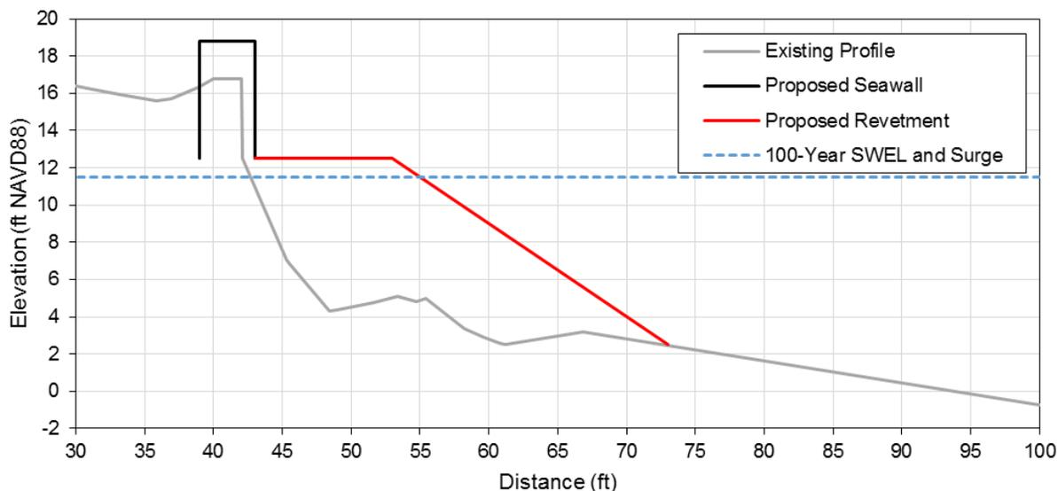
Figure 7.12 Schematic of proposed seawall and revetment design along Surfside Drive where the seawall height is increased by 2 feet and the fronting revetment is expanded.
