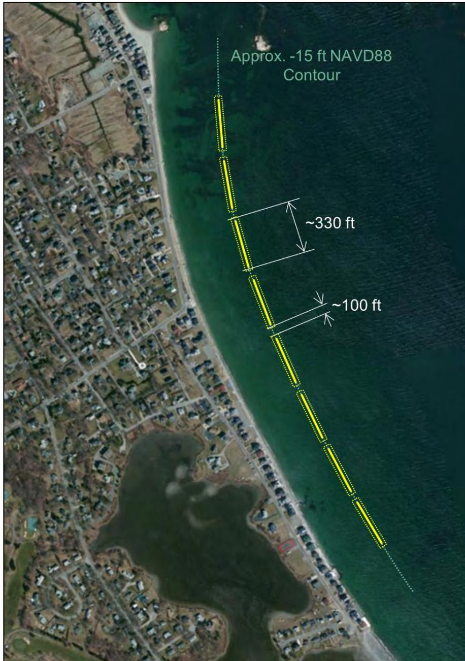
Figure 6.11 Approximate breakwater placement along the North Scituate Beach and Surfside Road shoreline. Dashed yellow outline shows the approximate footprint of the breakwater. This breakwater configuration was considered as a potential shore protection approach in the alternatives analysis for the North Scituate Beach Nourishment Project.
