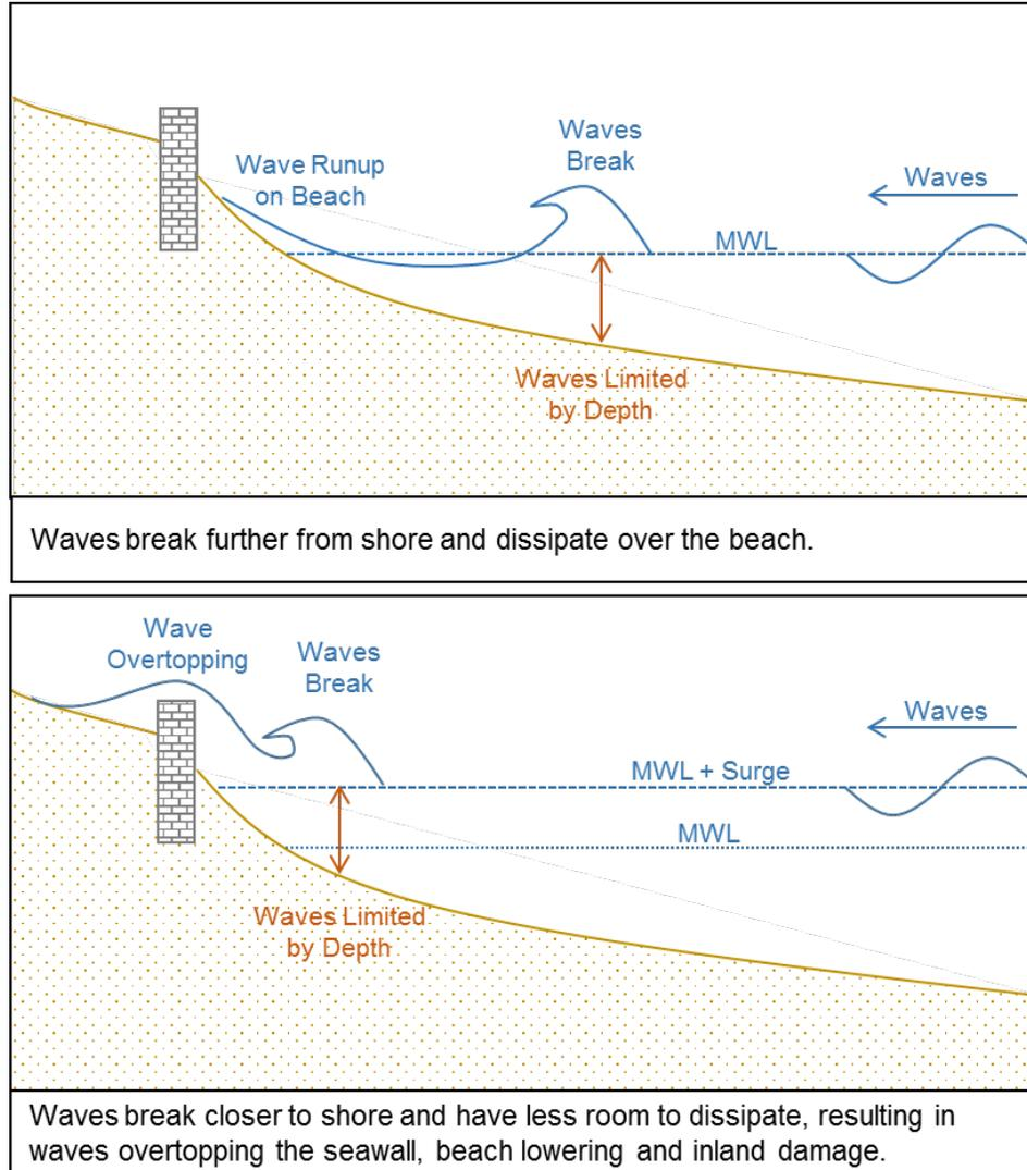
Figure 6.2 Effect of storm surge on wave and armored shorelines.
