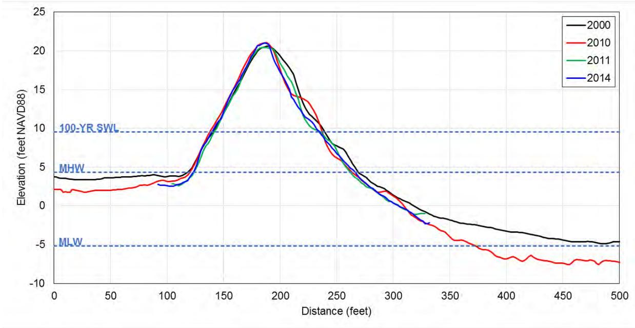
Figure 2.9 Profile change from 2000, 2010, 2011, and 2014 at Transect 1 (Mann Hill Beach). In addition to the LiDAR profiles, the dashed lines indicate the elevation of Mean Low Water (MLW), Mean High Water (MHW), and the 100-year Still Water Elevation (100-YR SWL).
