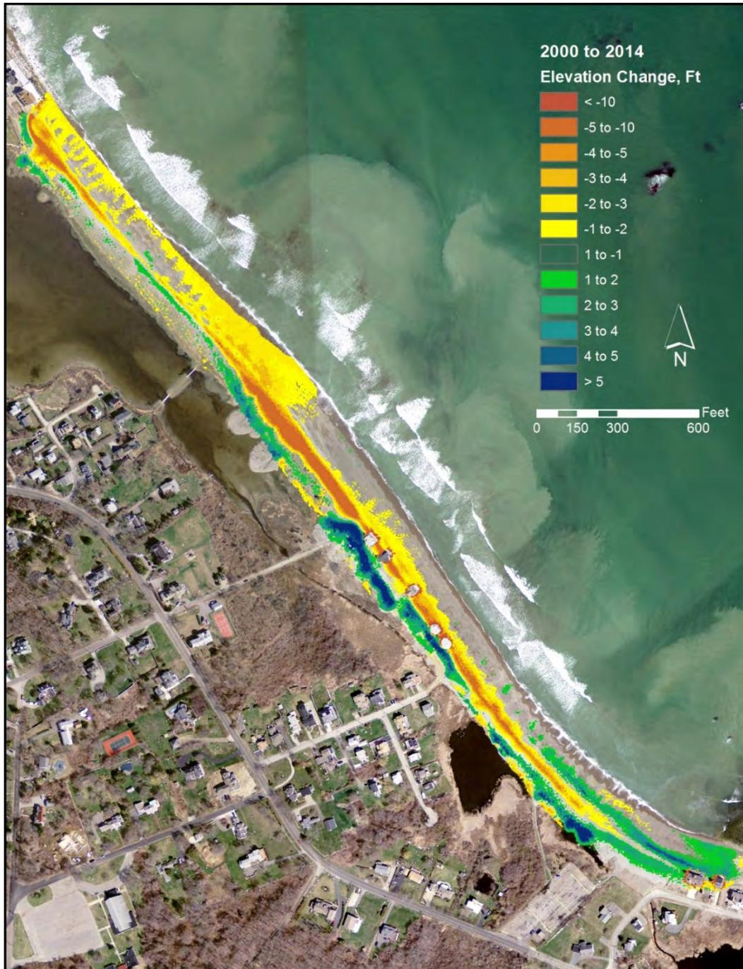
Figure 2.17 Topographic change from LiDAR data computed between 2000 and 2014 for Mann Hill and Egypt Beaches, where negative values indicate erosion and positive values indicate accretion.
