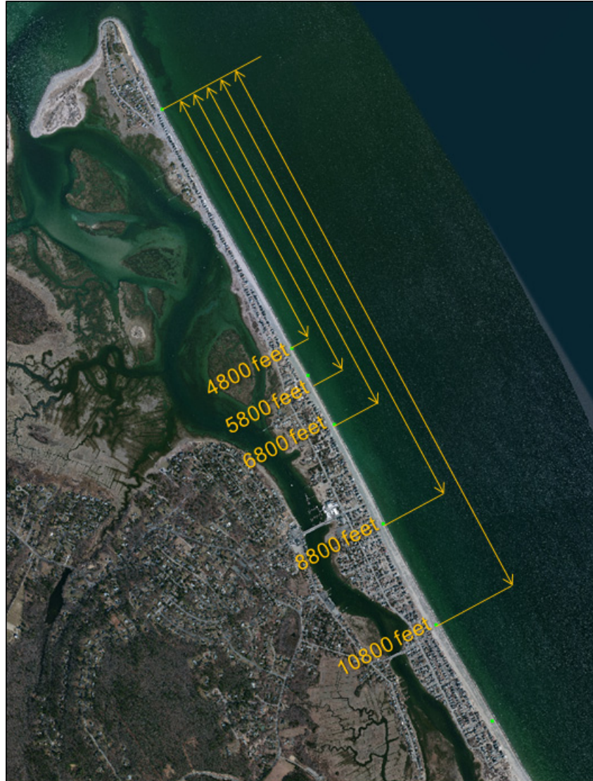
Figure 3.3 Modeled nourishment lengths along Humarock Beach starting at 10 Cliff Road South.
