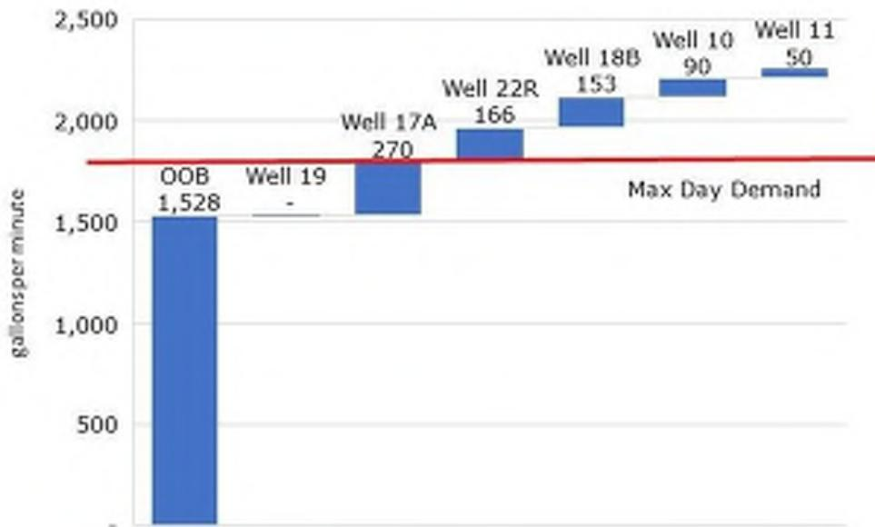
**Figure 2-22:** Current Production Capacity with OOB WTP Offline and Wells 17A and 18B Online (at Max Permitted Rate)
