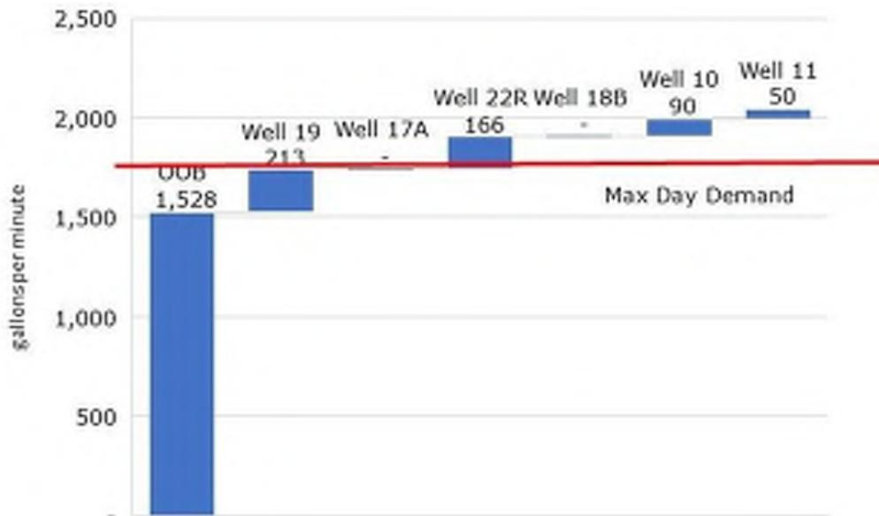
**Figure 2-21:** Current Production Capacity with Largest Well Offline (#19) and Wells 17A and 18B Online (at Max Permitted Rate)
