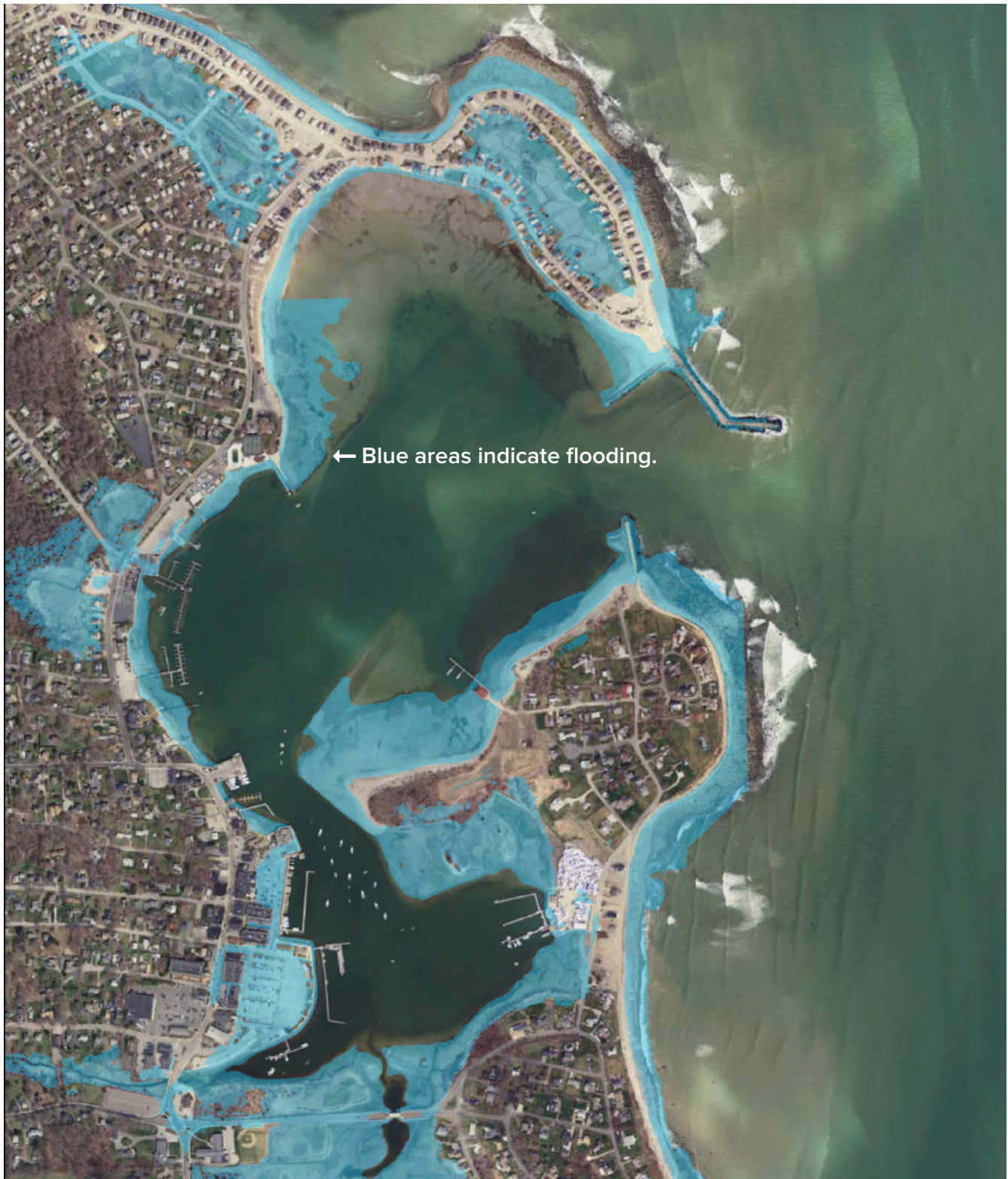
Figure 9. Flooding from Two Feet of Storm Surge in Scituate Harbor The areas in light blue show the present-day (2020) extent of flooding during a spring tide due to two feet of storm surge from a 10-year storm (a storm with a 10% probability of occurring in a given year.) This storm surge level is equivalent to the projected height of water during a spring tide on a clear day if the sea rises another two feet by 2070. (Applied Coastal, 2020)
