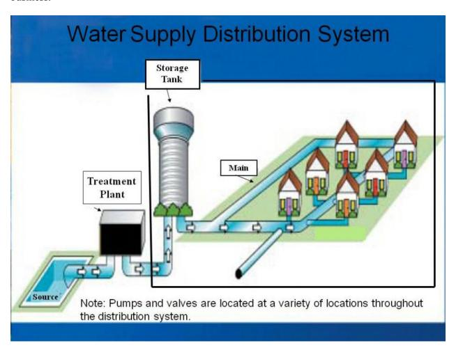
The distribution system is one cause of the brown water problem in Scituate. Years of inactivity in replacing system components such as old piping and a lack of a comprehensive flushing and maintenance plan has led to the build-up of years of sediment in the distribution system. This sediment, consisting mainly of iron and manganese, causes the discoloration of the water (brown
