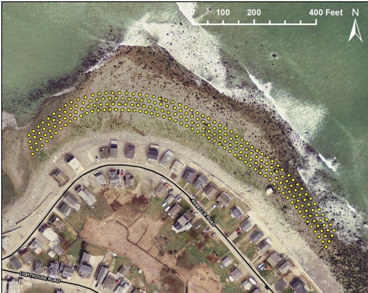
Figure 6.13 Configuration of individual boulders (represented by the yellow circles) forming a boulder dike along Cedar Point.
