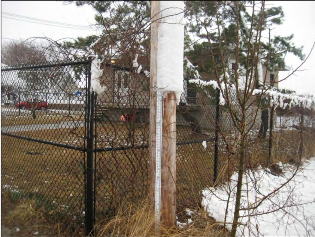
Figure 6.16 Flooding elevation is shown by the snow line at the Sand Hill pump station after Winter Storm Juno (photo by Jason Burtner, [www.mycoast.org](http://www.mycoast.org)).
